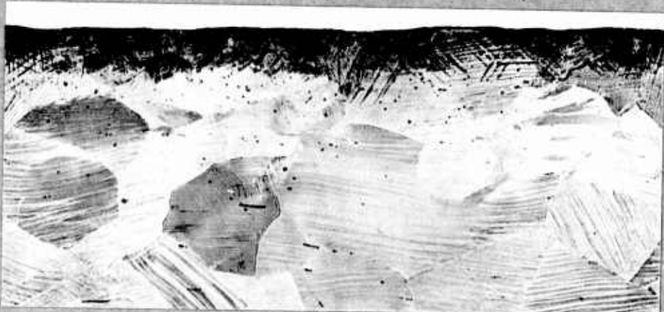
Nital Etch X250 Item A - Full hard (Rockwell C 40) - .0013" decarburization. Slip lines indicative of cold working - Poor ballistic characteristics.
