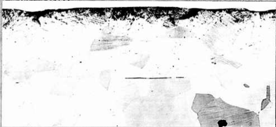
Nital Etch X250 Item B - Half hard (Rockwell C 30) - .0009" decarburization. Poor ballistic characteristics.
