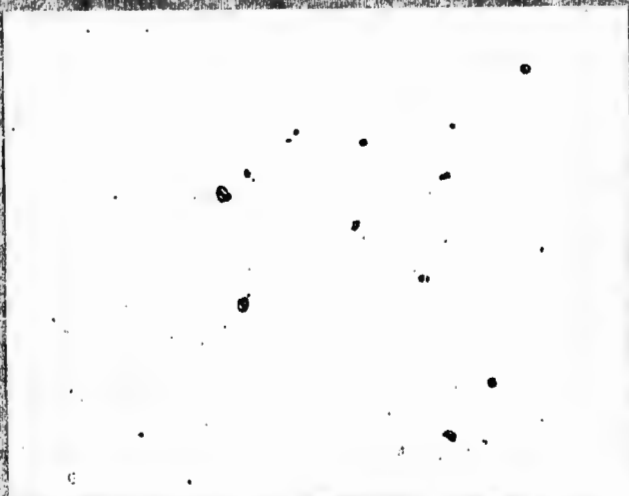
Plate 121. Unetched, Midwall. Typical also of plates Q115, Q123. Center. X100
