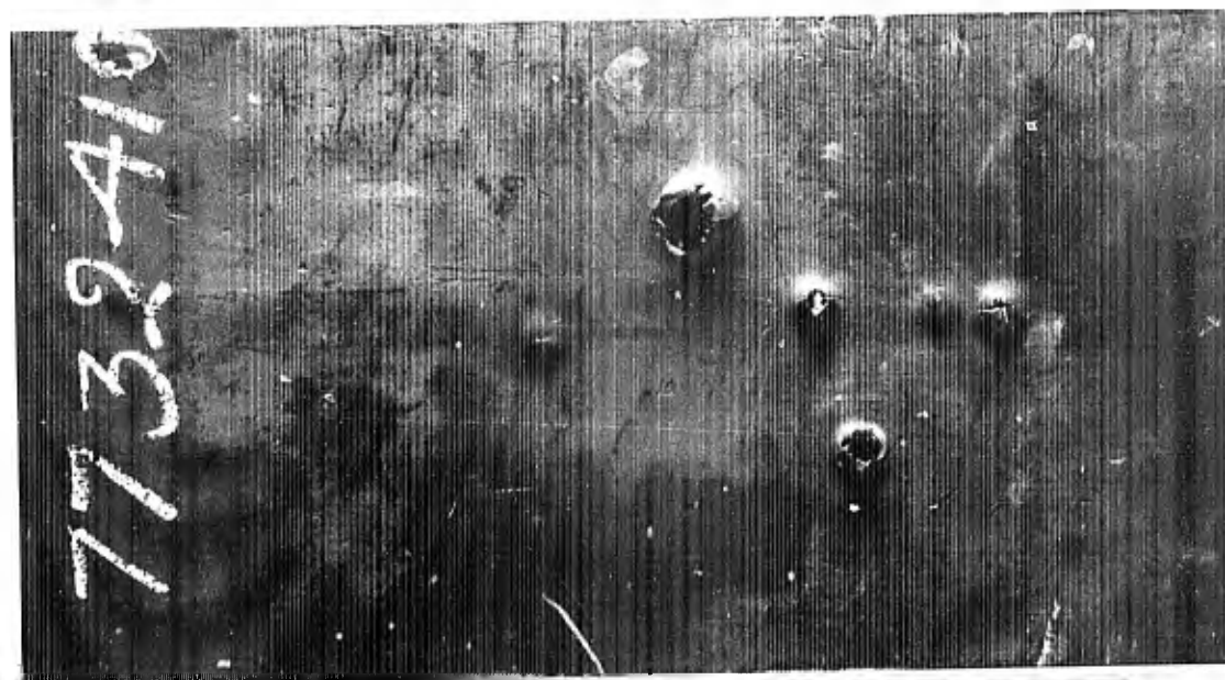
Fig. 212. Same heat as shown above but at the 410 Brinell level. Cross-section equiv. Brinell hardness 426. Ballistic limit 2360 F/s.
