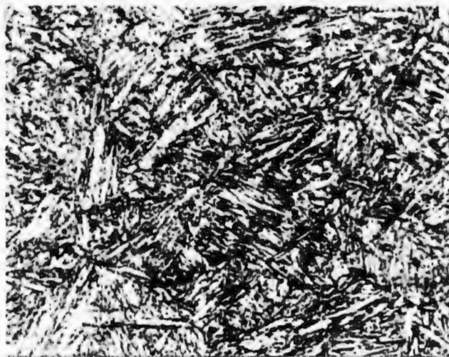
Picral Etch Plate 7 Plate 15 X1000 Tempered martensitic structures characteristic of plates 1, 3, 4, 7, 13 14 and 15.
