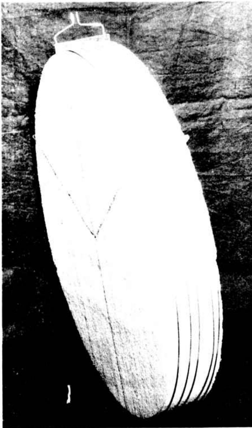
Fig. 5. Five-turn loop antenna.
