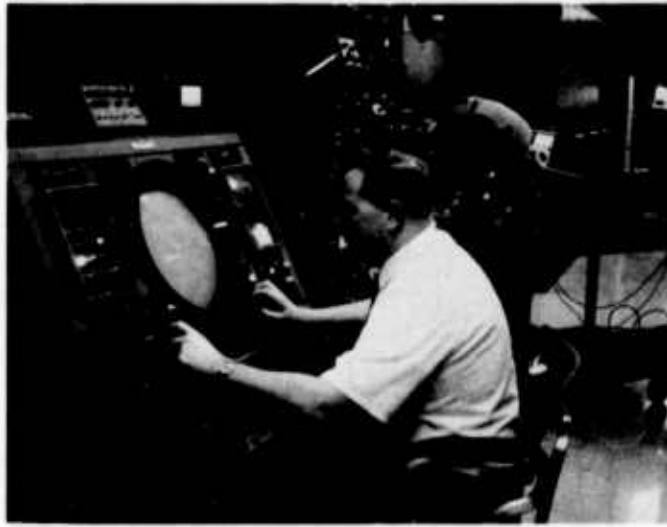
Figure B40. Air Route Surveillance Radar Display
