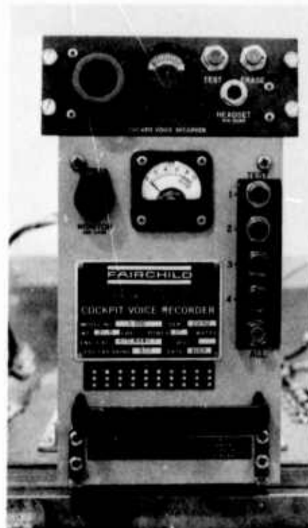
Figure B4. Cockpit Voice Recorder and Control Unit
