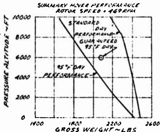
From this plot (Figure B), it can be seen that the 95 degree F hover ceiling at normal gross weight was determined to be approximately 3800 feet, an altitude substantially lower (37 percent) than the
