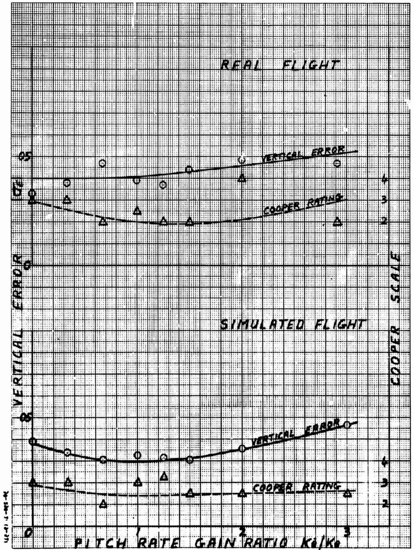
FIGURE 32 INFLUENCE OF ELEVATION RATE GAIN RATIO ON TRACKING AND COOPER RATING
