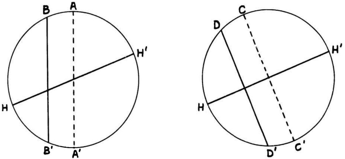
FIGURE 2 DISPLAYS WITH MIXED AND SINGLE AXES. Displacement from AA' to BB' shows heading in aircraft axes. Displacement from CC' to DD' along horizon HH' shows heading in earth axes.
