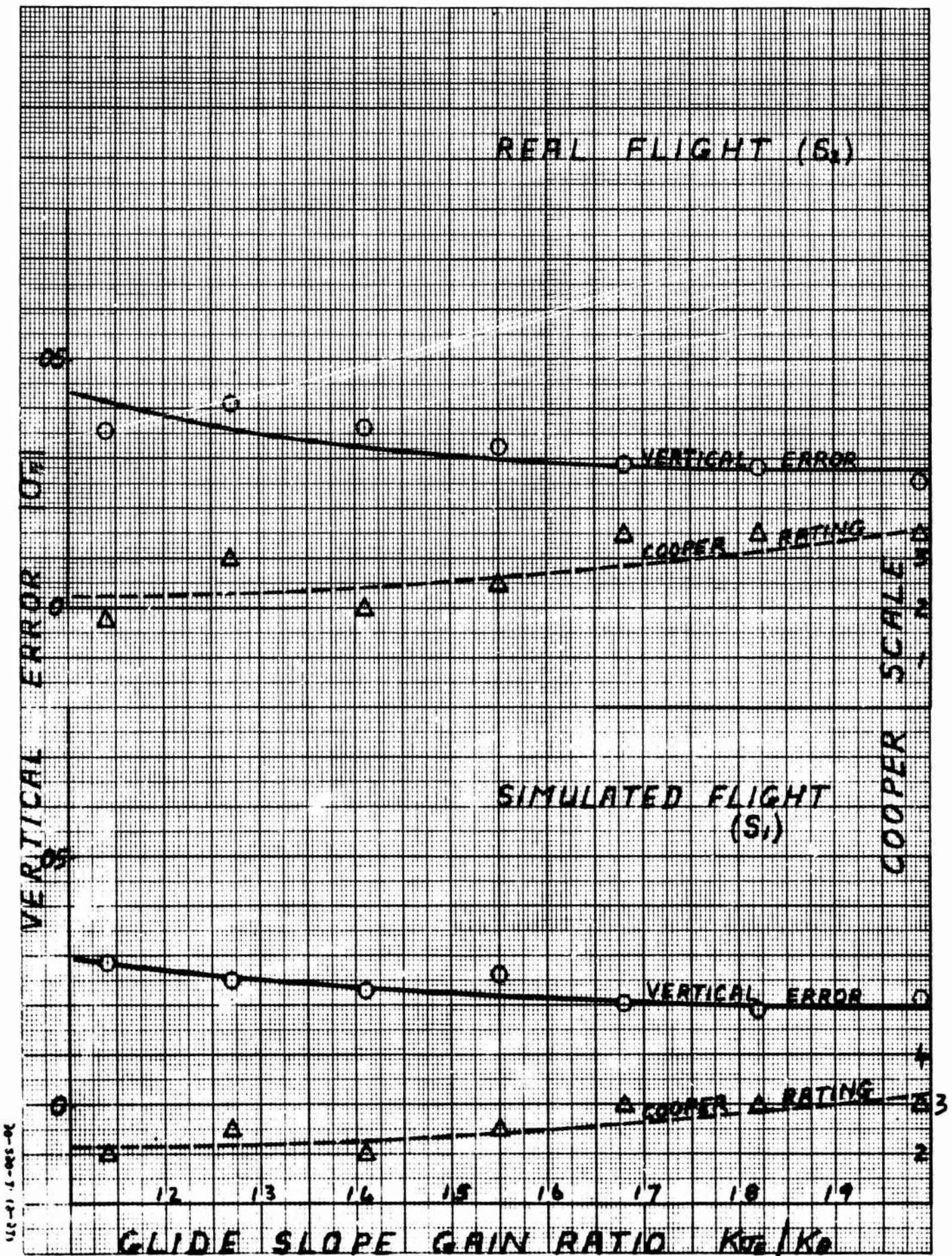
FIGURE 34 INFLUENCE OF GLIDE SLOPE GAIN RATIO ON TRACKING AND COOPER RATING
