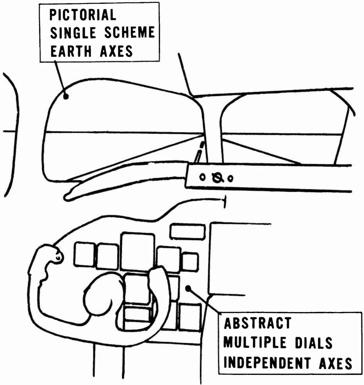
FIGURE 3 DIFFERENCE OF INTERPRETATIVE METHOD FOR INSTRUMENT PANEL AND FORWARD VIEW
