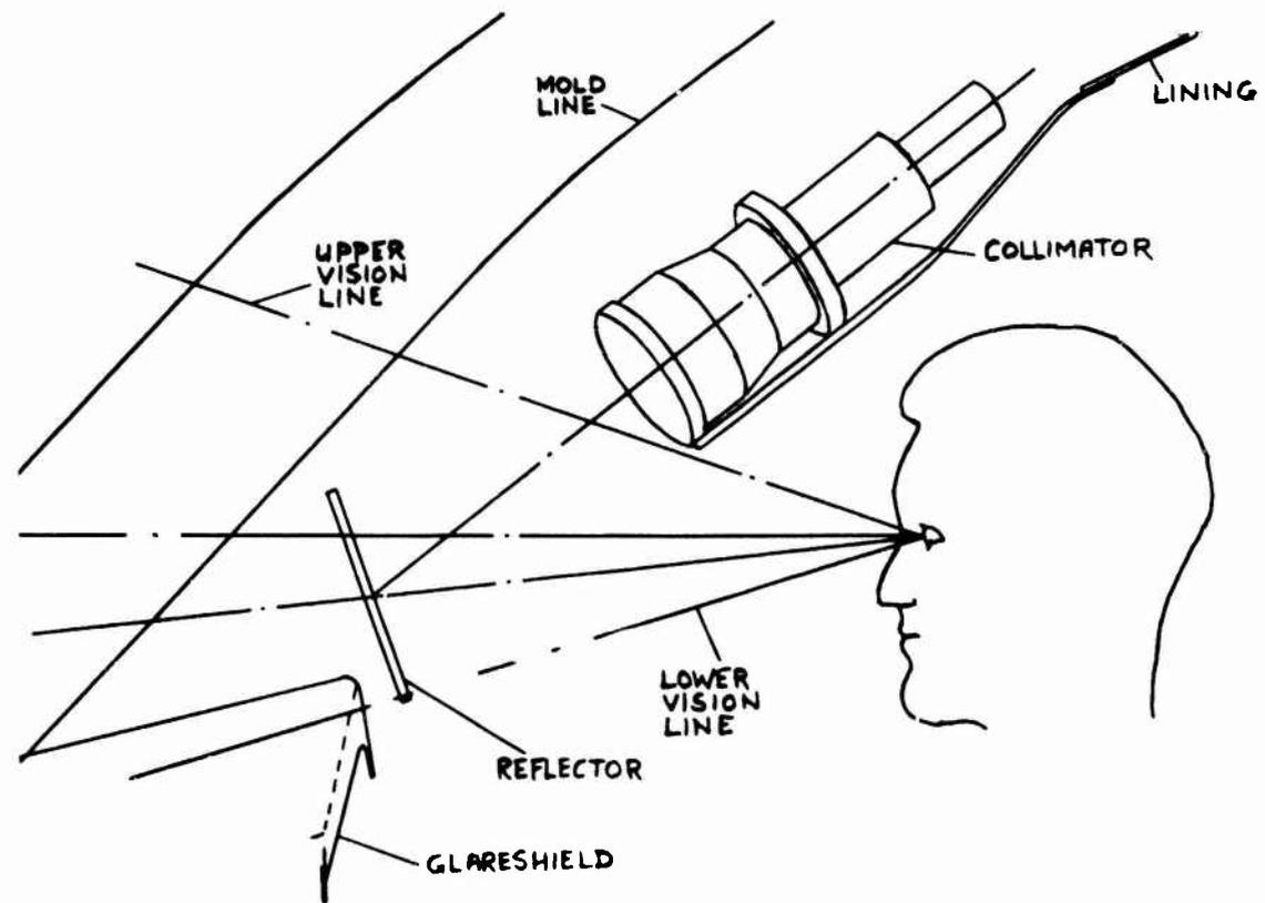
FIGURE 17 OVERHEAD INSTALLATION SHOWING HEAD CLEARANCE AND UNOBSTRUCTED WINDSHIELD
