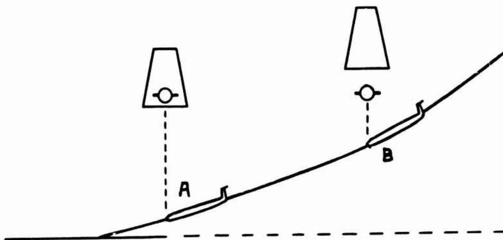
FIGURE 39 EFFECT OF BEAM BEND IN DISPLACING AIRCRAFT-STABILIZED SYMBOLS RELATIVE TO GROUND
