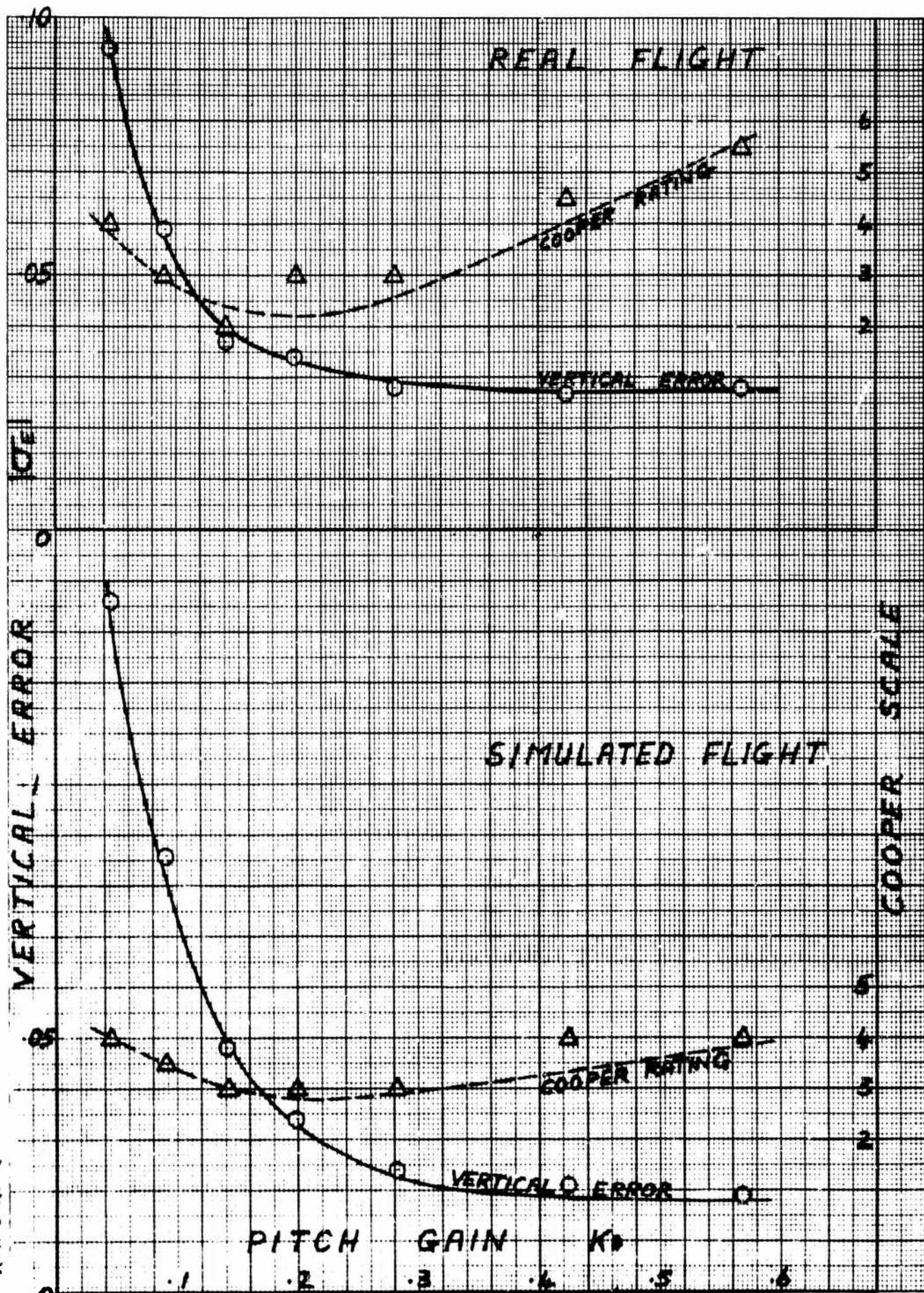
FIGURE 31 INFLUENCE OF ELEVATION OR PITCH GAIN ON TRACKING AND COOPER RATING
