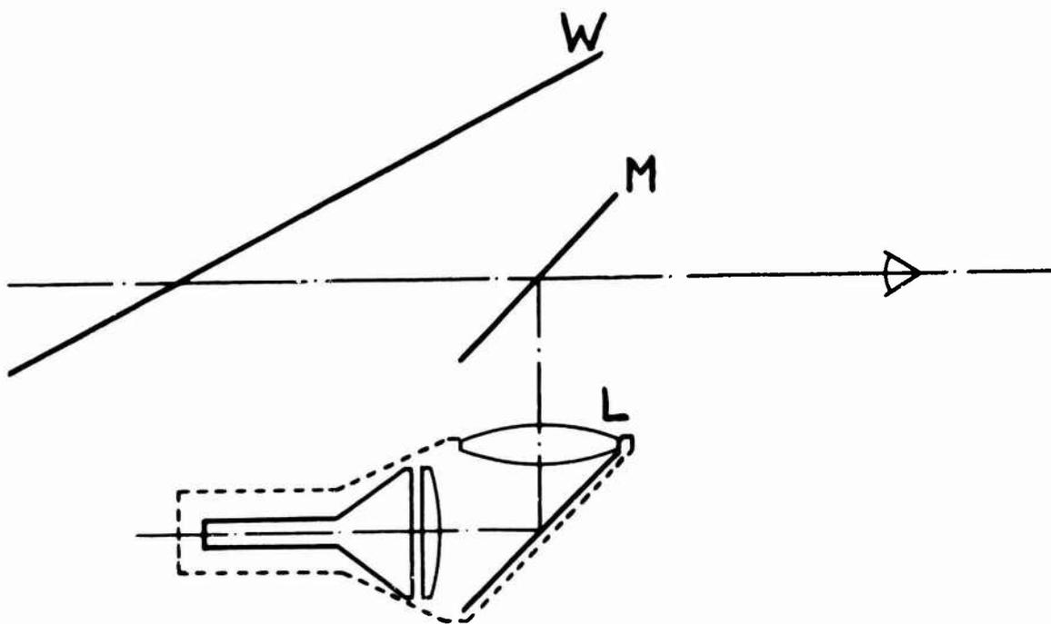
FIGURE 1 REFLECTING COLLIMATOR. Display superimposed on forward view through windshield, W, by partial mirror, M, and imaged at infinity by lens, L.
