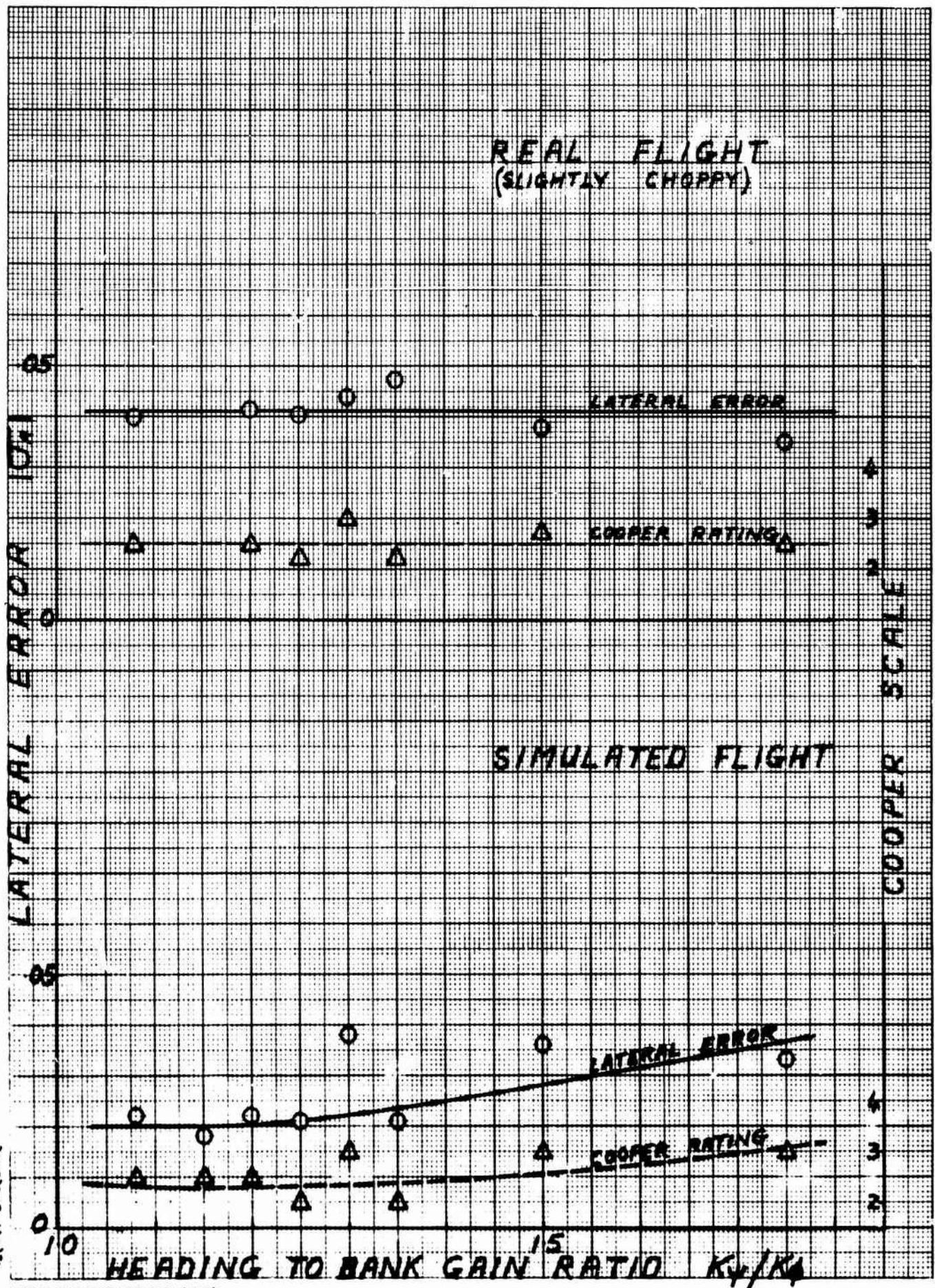
FIGURE 33 INFLUENCE OF HEADING TO BANK GAIN RATIO ON TRACKING AND COOPER RATING
