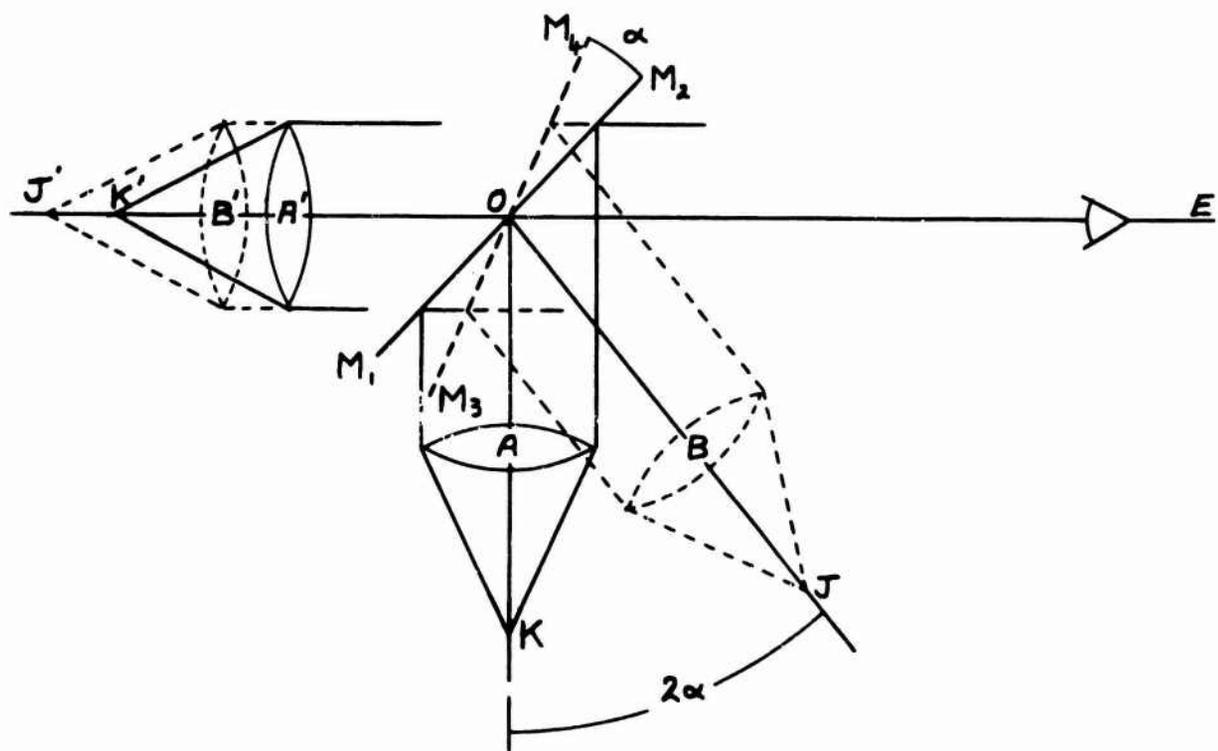
FIGURE 10 ORIENTATION OF REFLECTOR AND COLLIMATOR
