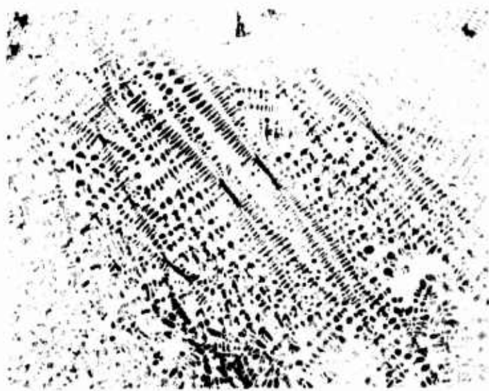
Figure 6. Dendritic structure of Fe-Ni-Cr alloy cooled at 1.15^{\circ}\text{F.} per minute. Water quenched just before complete solidification. 12X.
