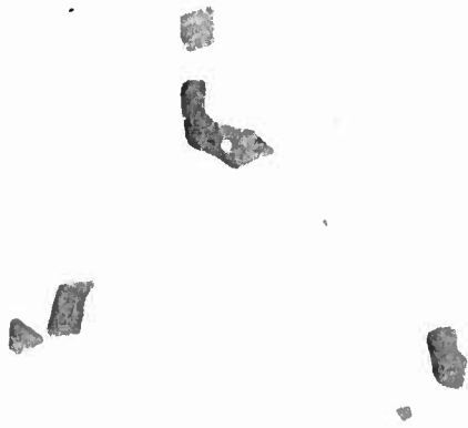
Figure 26—Type III inclusions, typical of the base steels AE-1, AE-2, AE-4. Unetched, 500X
