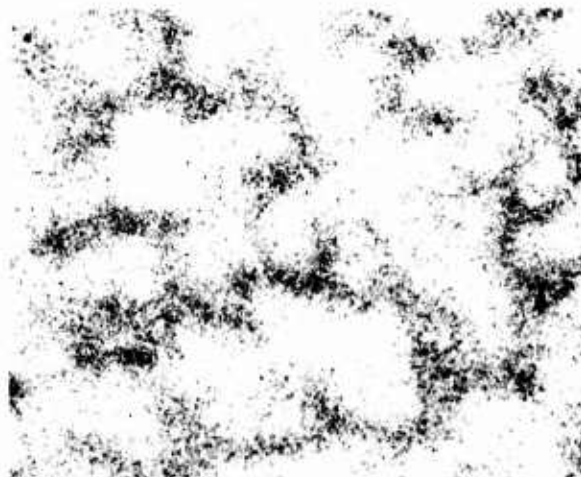
Tempered bainite and tempered martensite 4-inch section
