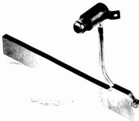
FIGURE 1: PARTING TOOL HOLDER W/TREPAN TOOL TIP AND OIL PRESSURE TUBE.
