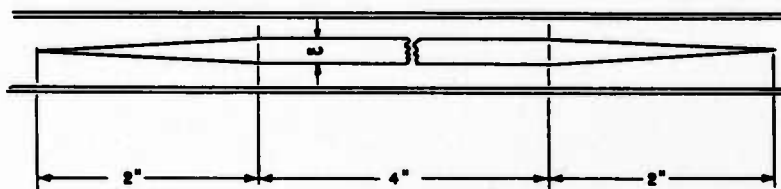
DETAIL OF SLOT IN MAIN GUIDE X BAND
