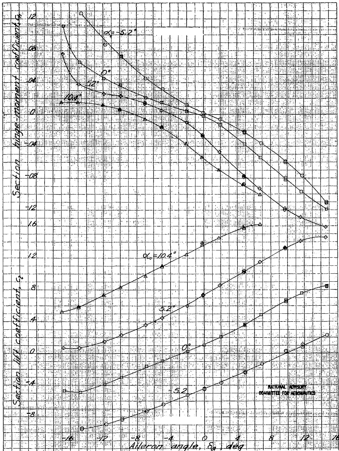
Figure 22. - Variation of section coefficients with aileron angle at various section angles of attack \alpha_o . Impact pressure q_o of 240 pounds per square foot. Data from two-dimensional tests in the Langley Stability Tunnel.
