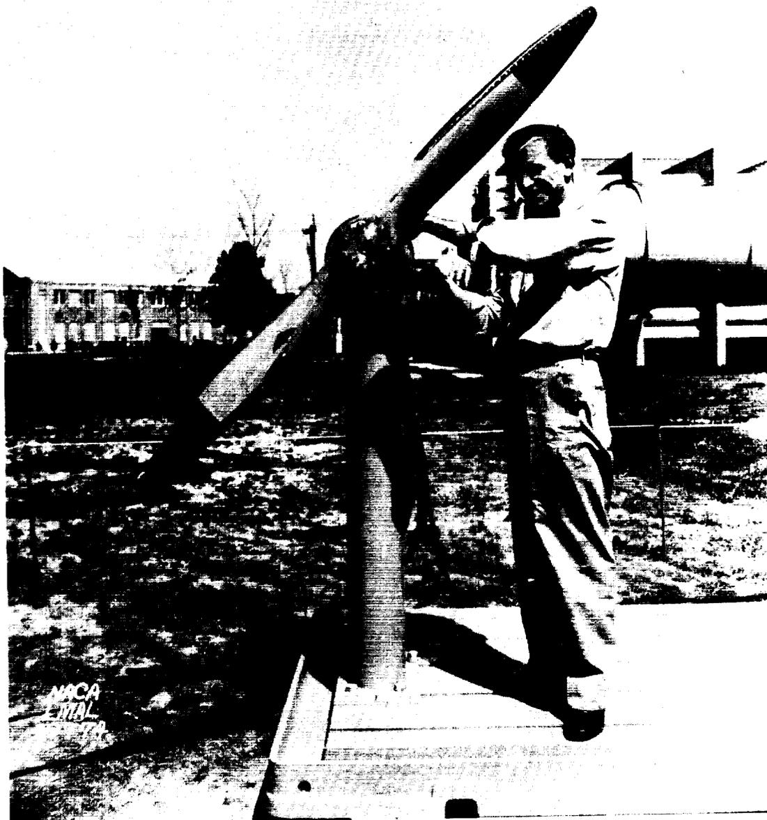
(b) Two-blade propeller mounted on test stand.
