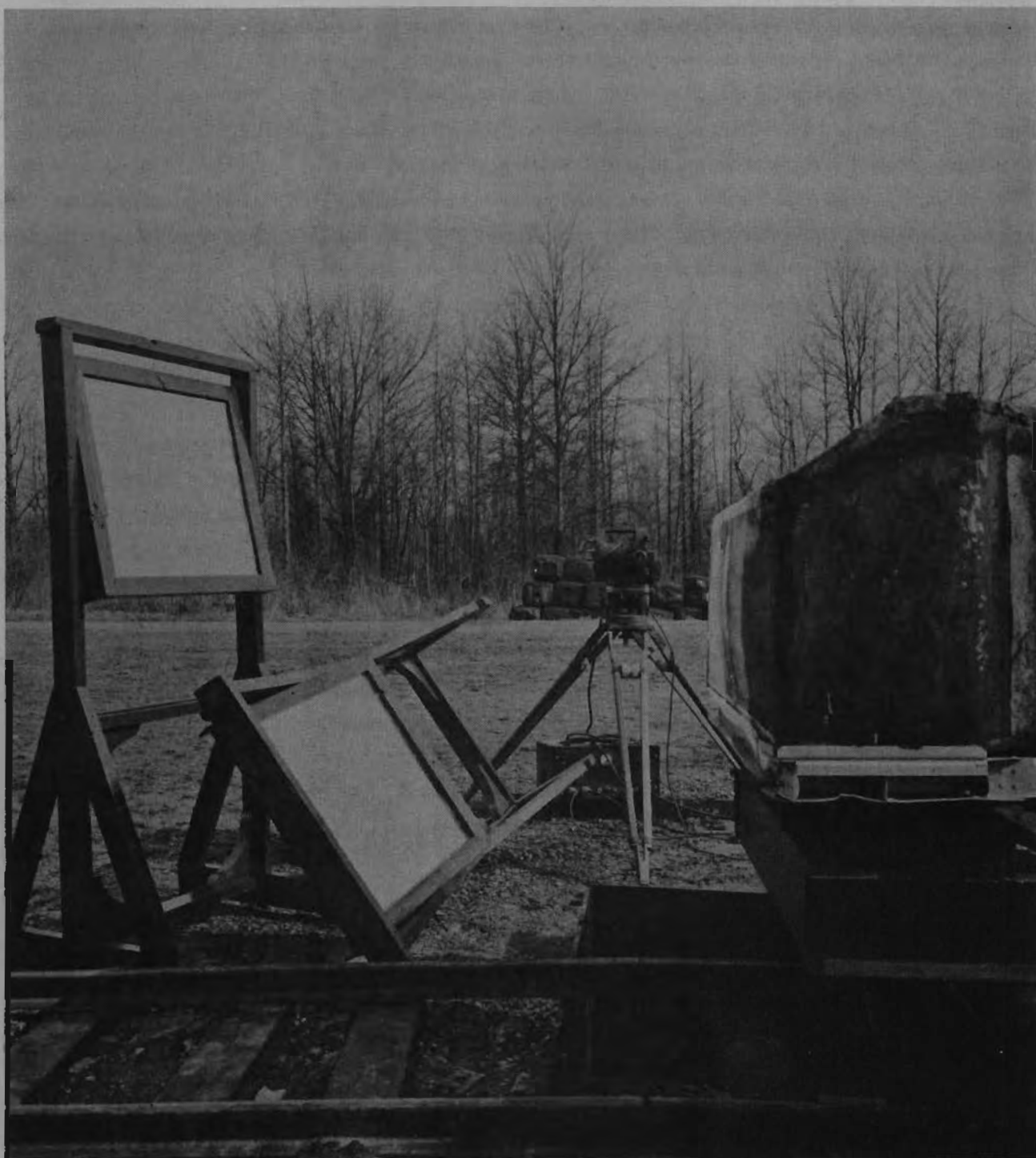
FIG. 29. Ultra-High Speed Camera Set-up for Photographing the After Effects of Bullet Entry into Fuel Cells. Mirrors are used to reflect sunlight onto the face of the fuel cells.
