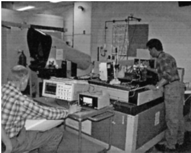
Figure 2 – Photograph of ultraprecision lathe in the Liner measuring configuration.
