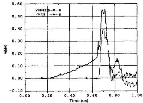
Figure 9. Prepulse suppression switch waveforms showing input and output.
