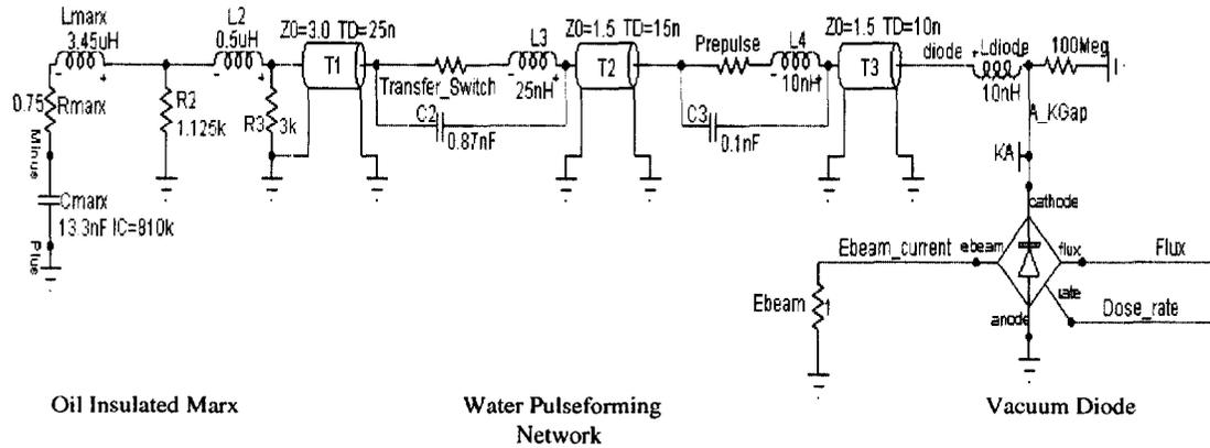
Figure 3. CXS model producing diode electrical input requirements.
