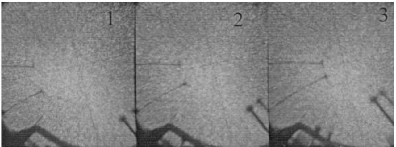
Figure 8: Shadowgraphs for three different times. Times increases from left to right. Micro-jets can be observed moving inward toward the center of the target assembly. Calibration cross hairs shown are 12 microns in diameter.
