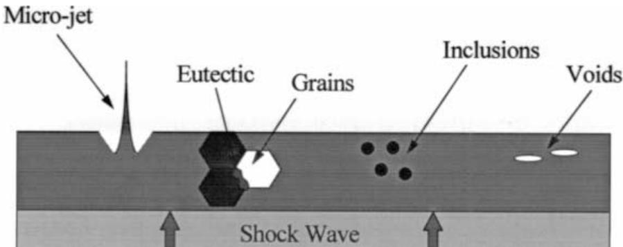
**Figure 1: Illustration of possible ejecta formation processes. The shock wave is shown coming from the bottom. The shock wave can interact in the material causing the material to break up and be ejected out ahead of the material.**
