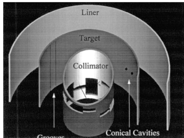
**Figure 4: Target assembly. The liner accepts current from the power flow channel and is driven radially inward and impacts the target. The collimator controls the number of particles that enter the center region.**
