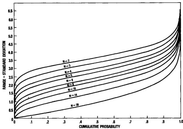
Figure 1. These curves relate the cumulative probability to the normalized range of pulse arrival times for  $N$  identical, simultaneously triggered switches. The numerical values are based on switch performance that can be described by a normal distribution with a standard deviation  $\sigma$ .
