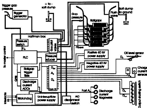
Figure 2. Block diagram of maintenance unit controls.
