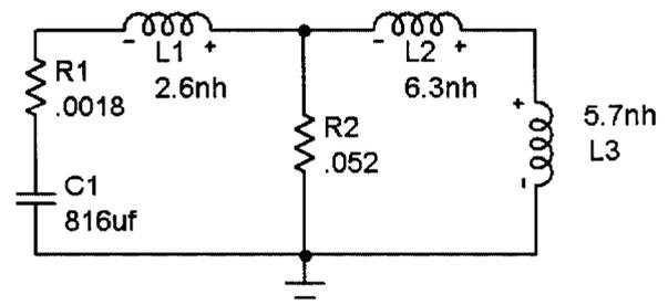
Figure 1a. Simplified Atlas schematic
