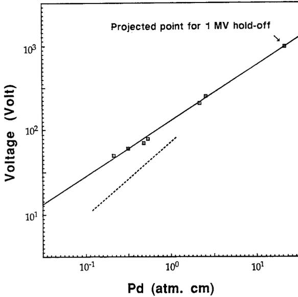
Fig. 4 Inpistron hold-off voltage ( $V_{ho}$  in kV) as a function of  $p \cdot d$  in atm-cm where  $p$  is the chamber pressure and  $d$  the gap distance.  $N_2$  gas is used for this test. Paschen curve for  $N_2$  of a single gap in uniform electric field is also shown with the dashed line for comparison.
