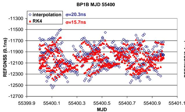
Figure 1. Comparison between the CGGTTS results obtained with either interpolation or Runge Kutta numerical integration, 4<sup>th</sup> order, for the TTS4 receiver located at the BIPM and connected to an H-maser.
