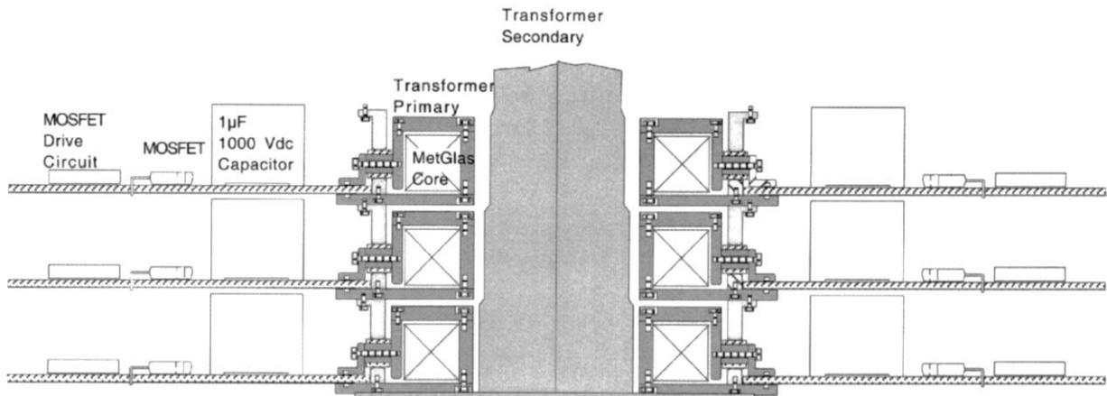
Figure 11. Cross-section of stacked modules making up an all solid state kicker pulser based on ARM-II technology.
