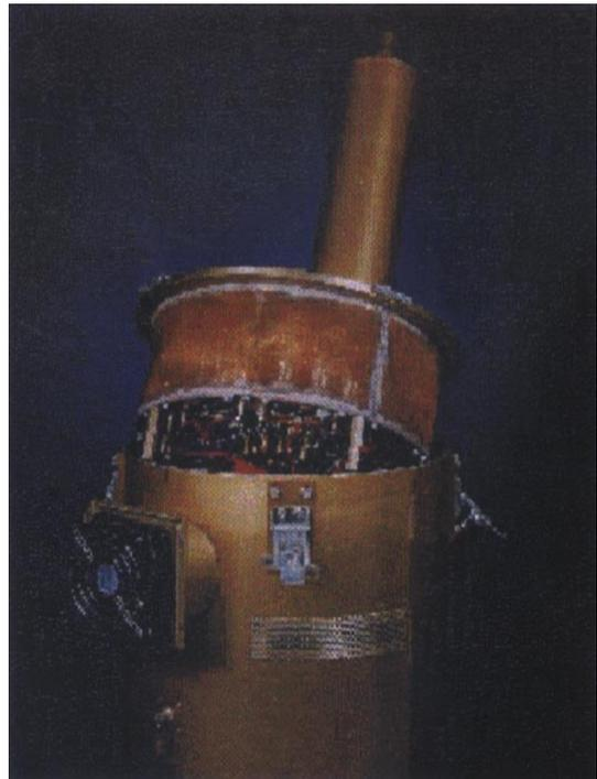
Figure 5. Photograph of the compact FET and planar-triode based fast pulser design.
