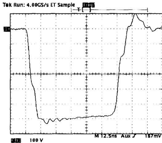
Figure 12. 60-ns pulsed response of partial FET assembly and core envisioned for an all solid-state kicker pulser.
