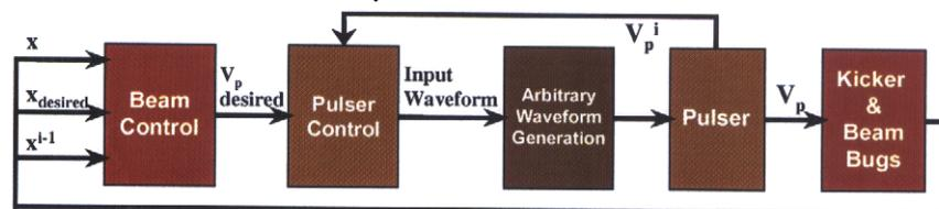
Figure 13. Flow diagram of pulser control logic for integrated beam/pulsers control.
