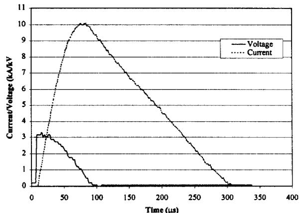
Figure 5. Current/Voltage output without inductor.
