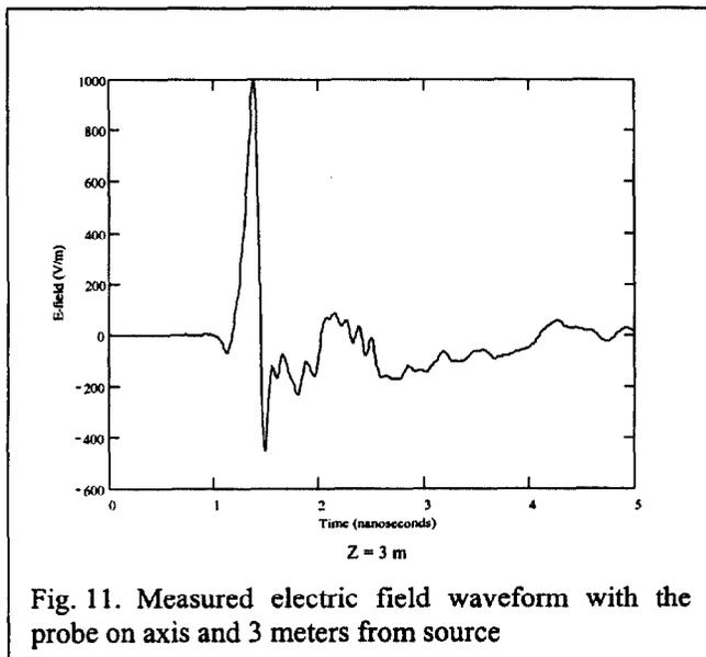
Fig. 11. Measured electric field waveform with the probe on axis and 3 meters from source
