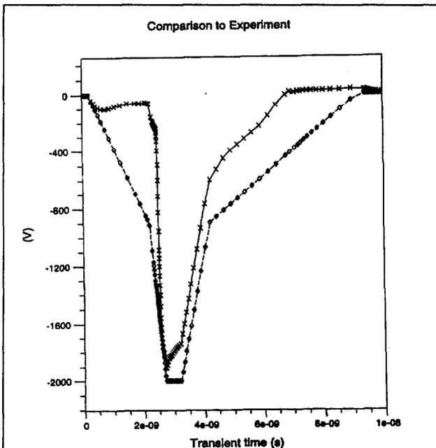
Fig. 3. Simulation of delayed breakdown in silicon
