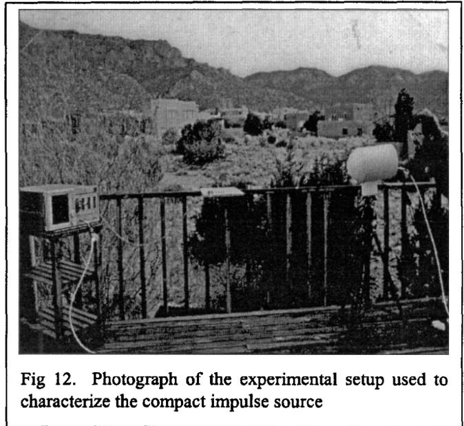
Fig 12. Photograph of the experimental setup used to characterize the compact impulse source
