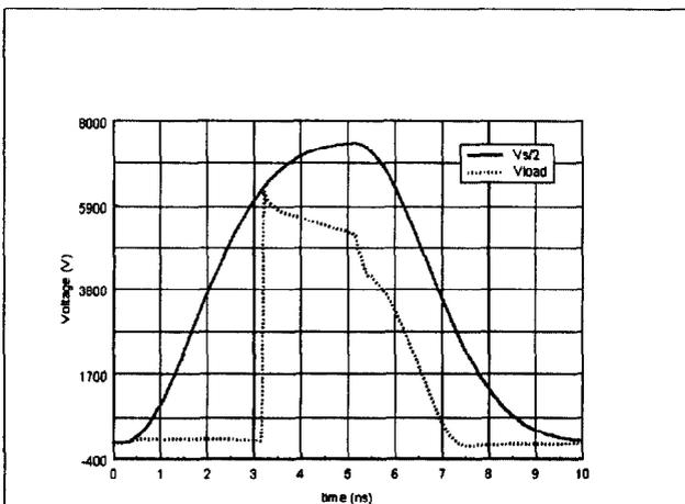
Fig. 4. Simulation of SiC device shows  $\Delta V = 6.2$  kV,  $\Delta t = 50$  ps, and  $dV/dt = 1.24 \times 10^{14}$  V/s.
