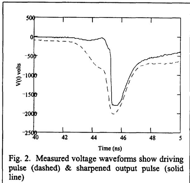
The University of New Mexico School of Electrical Engineering recently evaluated DBD switching technology by testing Russian DBD devices.[3,4] Commercial silicon devices have also demonstrated
