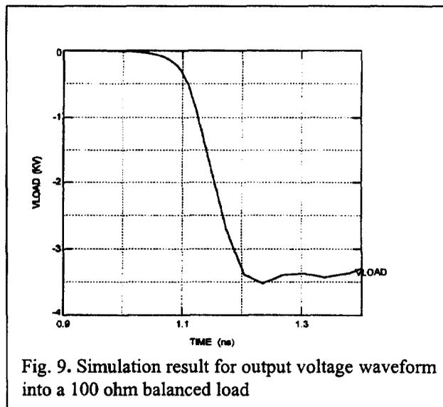
Fig. 9. Simulation result for output voltage waveform into a 100 ohm balanced load
