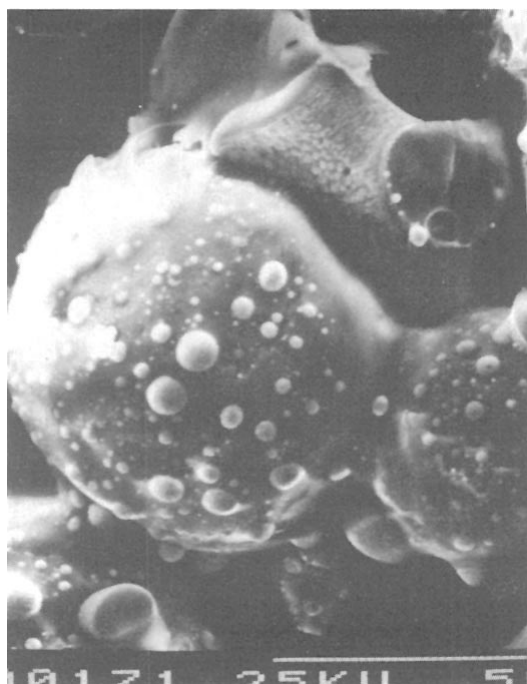
Figure 4. Scanning Electron Micrograph of copper/glass switch showing smaller droplets and neck between glass spheres. Marker indicates 50 \mu\text{m} .
