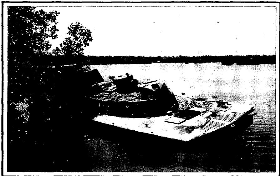
A knocked-out Japanese armored boat in the marginal swamp of SILUT LAGOON near LILOAN, CEBU. Craft was of metal construction with a wooden deck.
