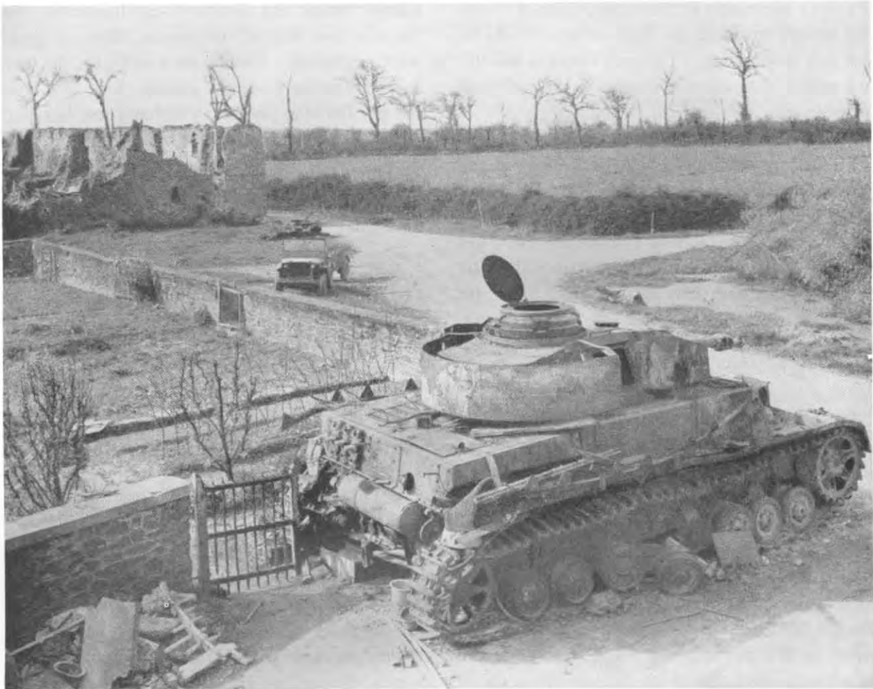
GERMAN MARK IV TANK, with a 75-mm gun, knocked out at le Mesnil-Durand in frontline fighting, while attempting to stop the drive of the 30th Division along the ridge. Note the strip of flashing around the tank's turret, as added protection against small-arms fire.
