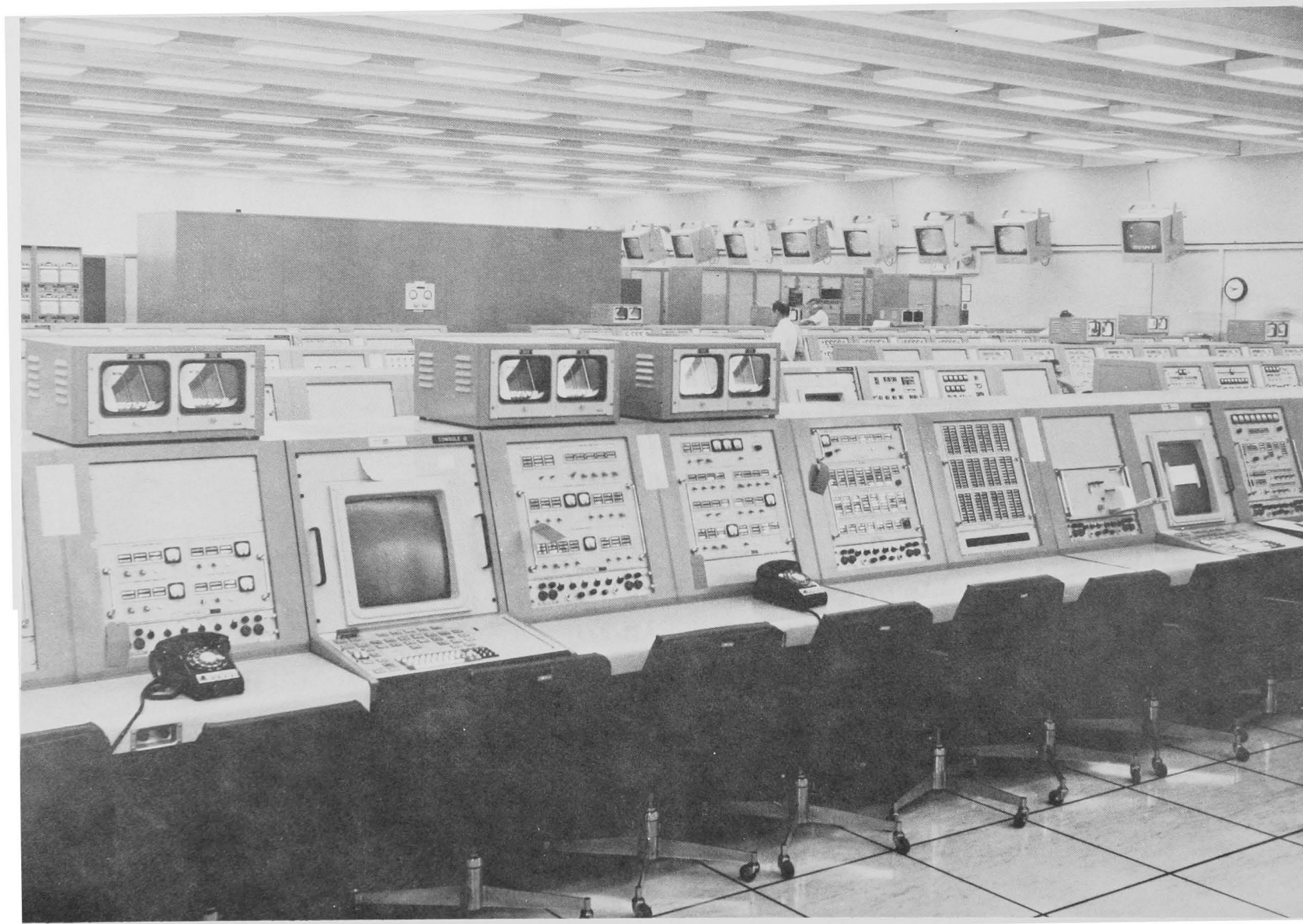
Interior of Firing Room 1, Launch Control Center, indicates complexity of console operation. Note console-mounted and wall-mounted television monitors.
