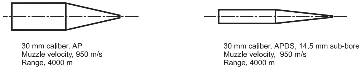
Figure 4. Automatic weapon 30 mm rounds are shown. Both are armour piercing projectiles. The full-bore projectile (left) is the same diameter as the APFSDS rod above. The hard-kill system has to distinguish by differences in velocity. The sub-bore projectile (right) is virtually as effective as the full-bore version but more difficult to detect.
