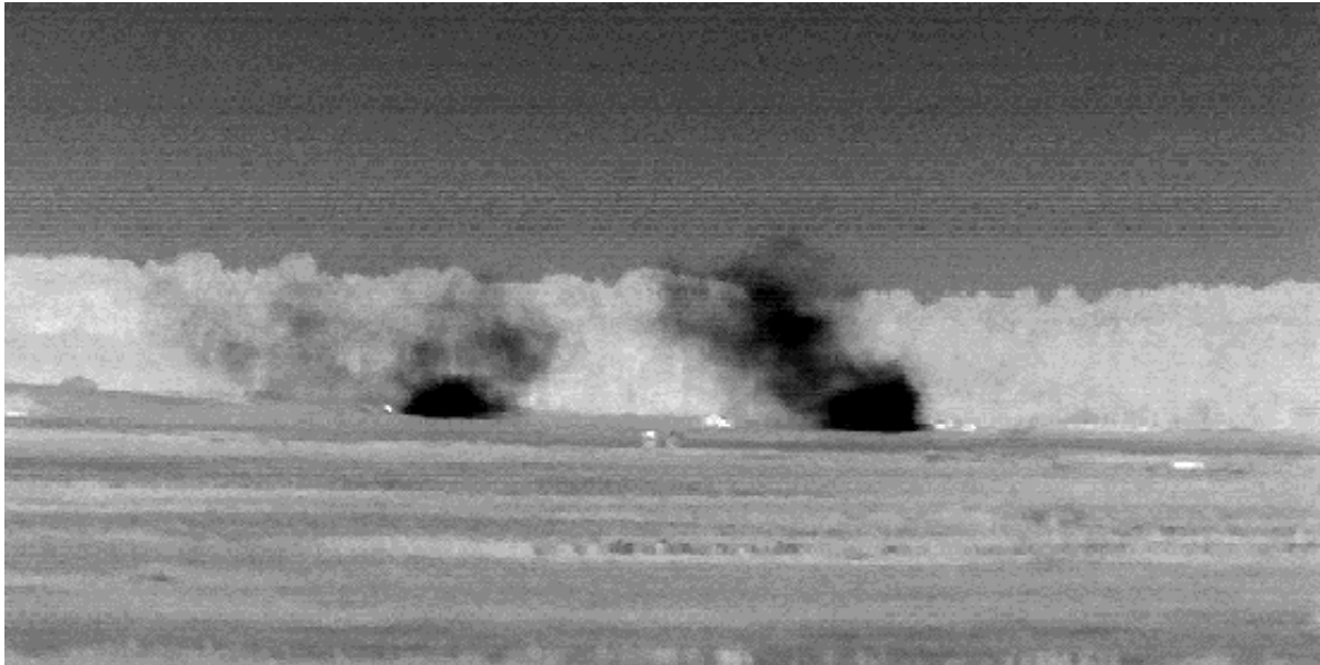
Figure C2. Static Scene: containing the 4 basic components: ultra-spectral terrain, vehicles corrected for range, battlefield obscuration and atmospheric transmission.
