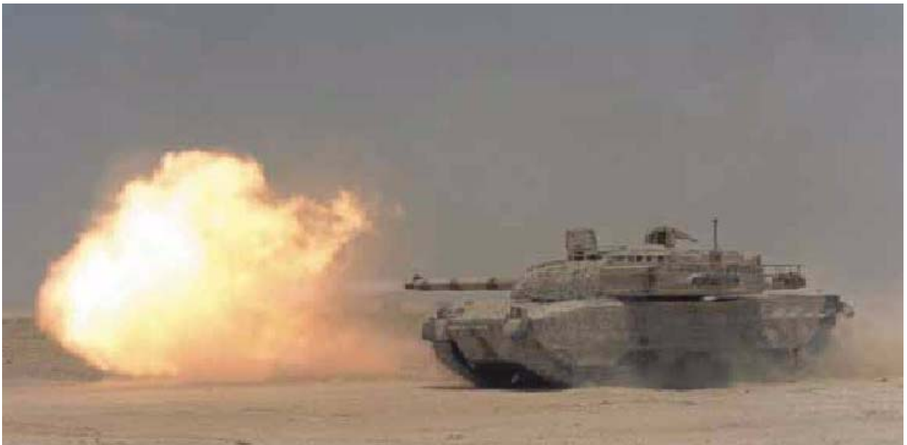
Figure 10. Typical muzzle blast produced by a 120 mm tank round fired by a Leclerc main battle tank. The vehicle hull is 6.88 m long and the height to the turret roof is 2.53 m.
