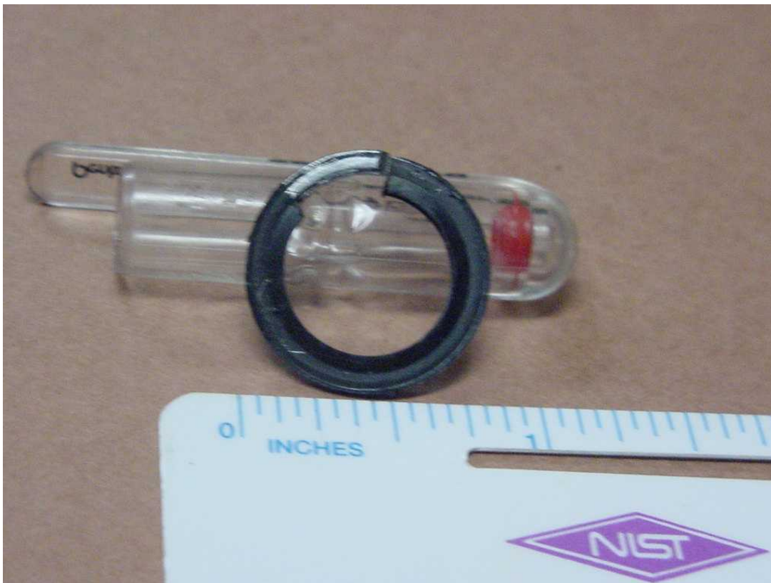
Figure II-8. Nitrile Encapsulated Steel Fuel Gallery Seal/Washer Used in the Bosch Pump
