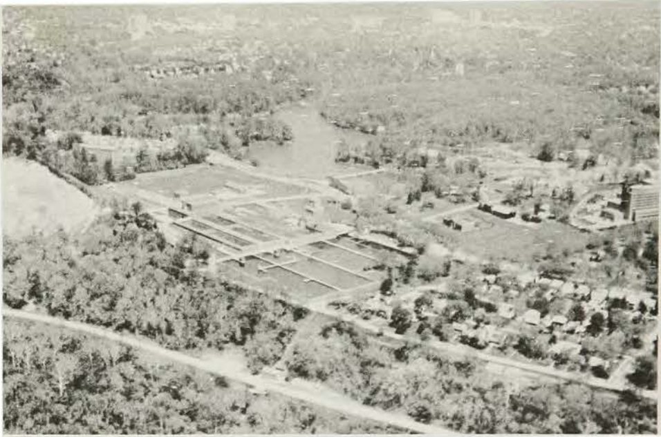
Aerial view of the Dalecarlia water plant. Water from Great Falls conduit enters forebay, upper center, and is then chemically treated and filtered.
