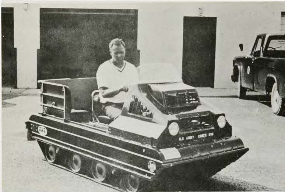
Above; Head Dam Operator Bert M. Smith demonstrates the PPT all-season vehicle used to reach remote parts of the reservoir. Machine, made in Quebec, has a maximum speed of 35 m.p.h.
