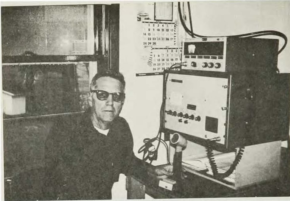
Present (1974) head damtender is Herbert C. Fox. Larger transceiver is a Communications Associates 27-B. Upper unit is a Sideband Associates Model 301.
