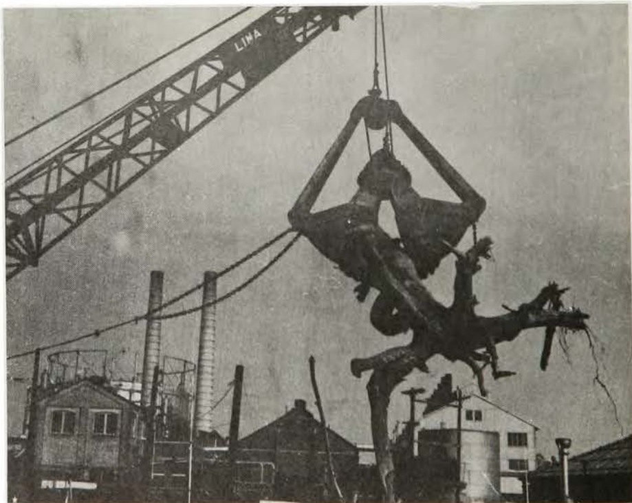
Drift collectors bring drift material to dock in Washington where it is removed from barges by this crane.
