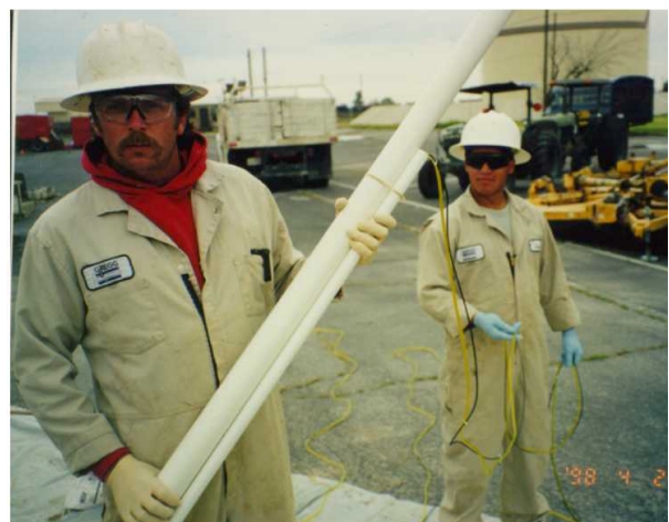
Photo 5. Attachment of sensor to PVC casing.
