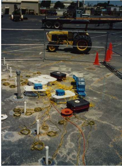
Photo 10. Site overview showing VW, VMPs, and data acquisition system.
