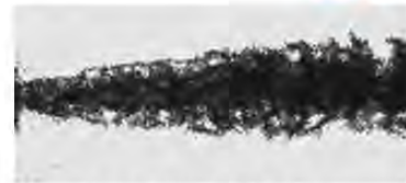
ballistic image of a diesel spray (Linne et al 2006, Exp. Fluids )
