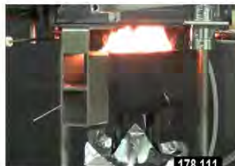
ASTM E662 @ 178 seconds - Core Material O
