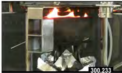
ASTM E1354 @ 300 seconds - Core Material G
