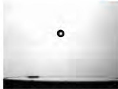
impact of a 3 mm water drop on a 2 mm water film (Guildenbecher et al, 2013, Exp. Fluids .)
