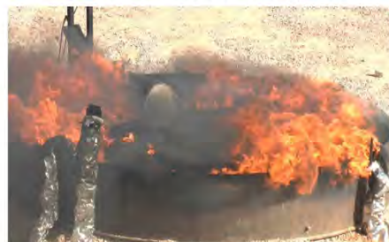
Rubble fire involving 900 lbs. of composite material and 320 gal. of jet fuel
