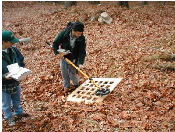
Figure 7-2. Cued identification of anomalies using an EM-61HH and template.
