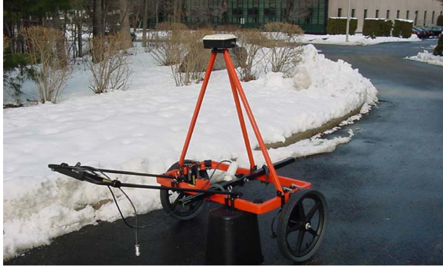
Figure 3-17. Dual-mode Man-Portable Simultaneous EMI and Magnetometer System (MSEMS) currently under development. Magnetometer is located in the center of the coil of the EM61 (SAIC 2006).
