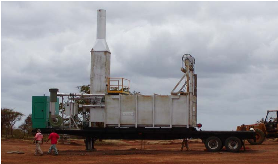
Figure 10-5. El Dorado Engineering flashing furnace for treatment of range scrap.
