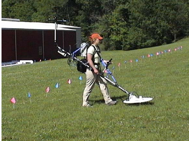
Figure 7-7. Dual-mode sensor survey at ERDC Vicksburg Test Facility.
