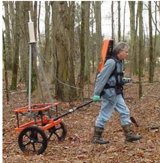
Figure 3-24. A local radio frequency navigation system integrated with an EM61.
