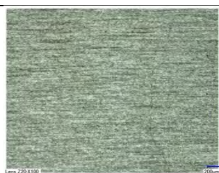
Figure 4-19 100X Intact SS-304 Coupon Surface
