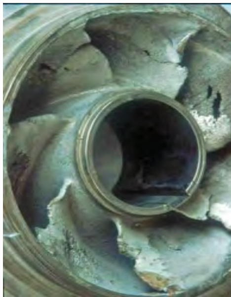
Figure 2-1 Example of Cavitation Erosion on a Pump Impeller
