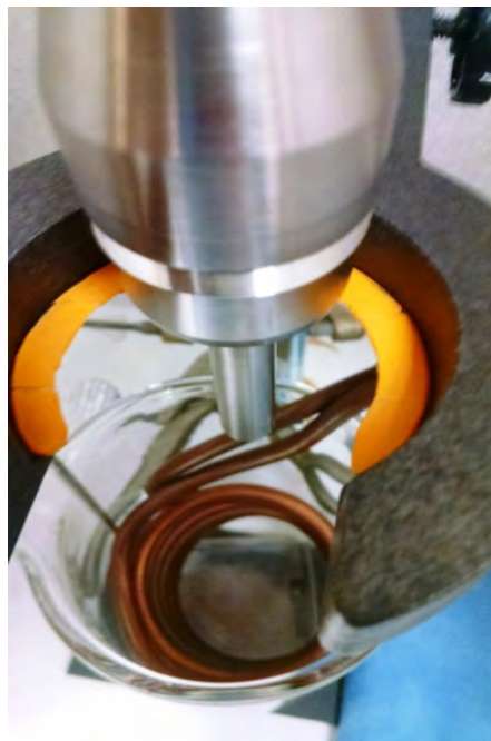
Figure 3-3 Close-up of 1-mm Orange Spacer Seated on Rim of Probe Clamp
