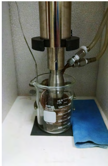
Figure 3-2 Close-up of Cavitation Erosion Test Setup
