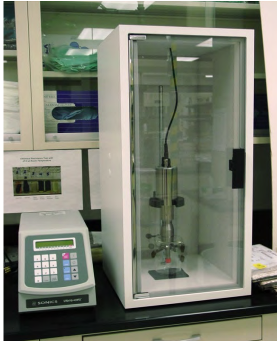
Figure 3-1 Setup for the Laboratory Cavitation Erosion Testing of Coupons
