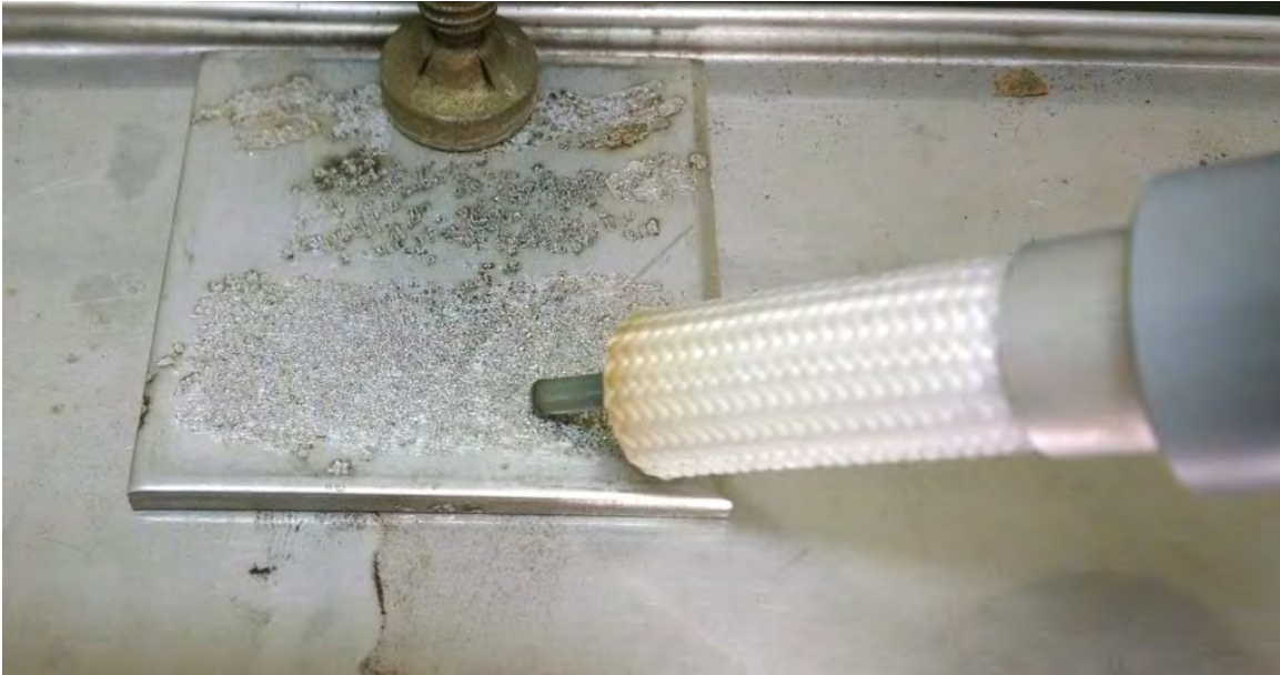
Figure 2-2 Close up of ESD Applicator Electrode at Substrate Surface
