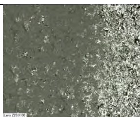
Figure 4-17 100X Edge of Fully Eroded Area of ESD Nitinol
