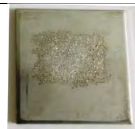
Figure 4-14 Cavitation Eroded ESD Stellite (slightly silvered area)
