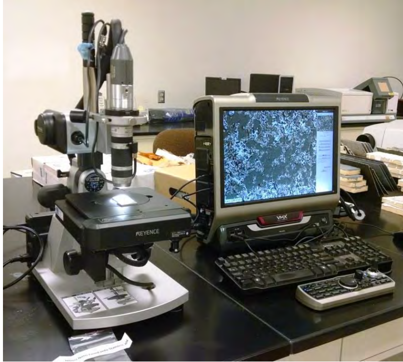
Figure 3-4 ESD Deposit Being Analyzed by Microscope
