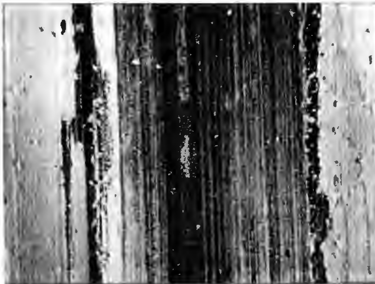
Figure 29. C71500 Copper-Nickel Wheel/ Rocklinized 316 Stainless (10X)
