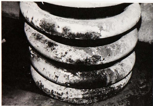
NORAD Spring, Showing Corrosion Effects
