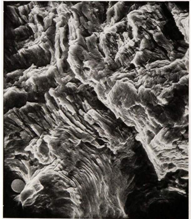
Metal Fatigue in Steel as Seen Through Scanning Electron Microscope
