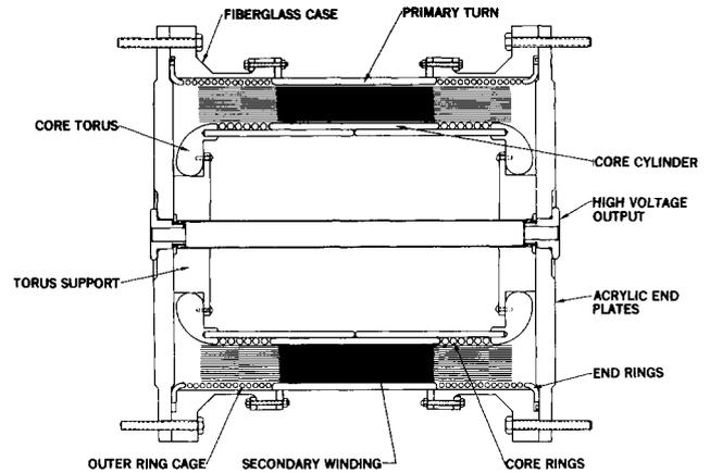
Fig. 5. Pulse Transformer
