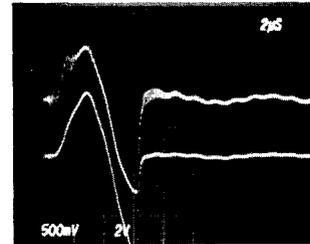
Figure 8. Secondary voltage waveforms from capacitive (top) and resistive (bottom) monitors
