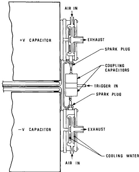
Figure 3. Two-section spark gaps
