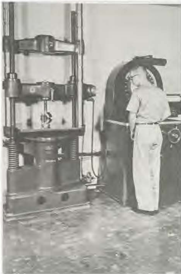
Marshall stability test in progress
