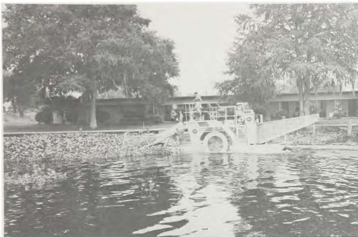
Mechanical harvester tested for waterhyacinth control in the St. Johns River, Florida
