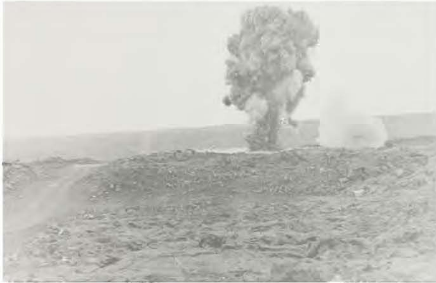
Smoke and volcanic dust billow in the air as two 40-pound charges are detonated over a lava tube located on the flank of giant Mauna Loa Volcano on the Island of Hawaii on 24 May 1976
