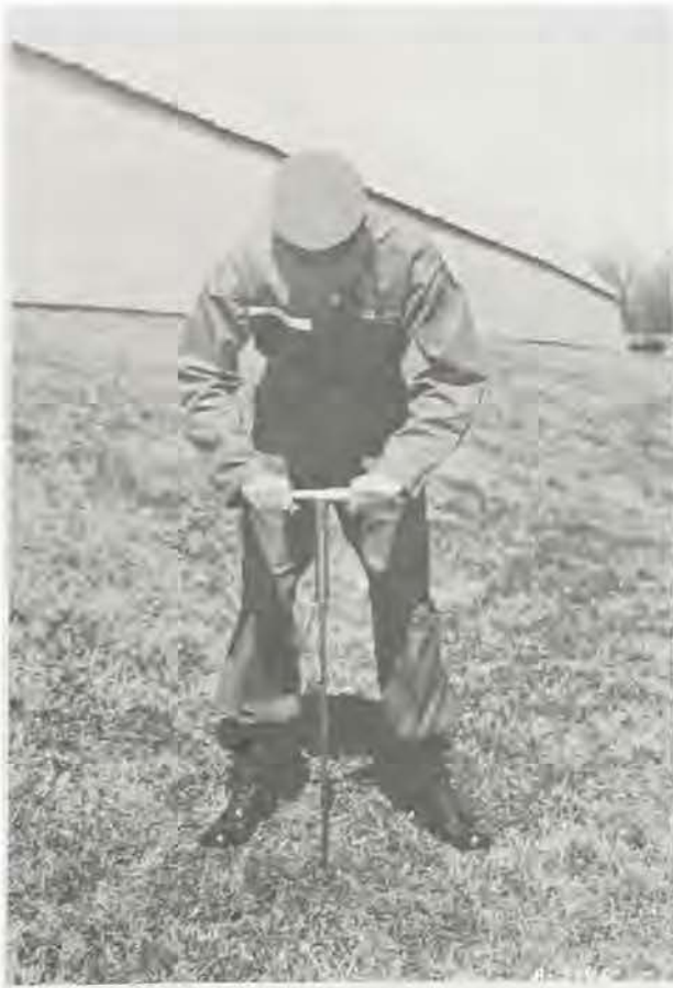
Cone penetrometer in use
