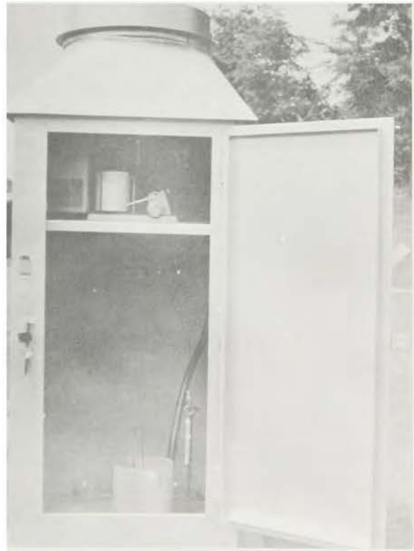
Inside of special type recording rain gage
