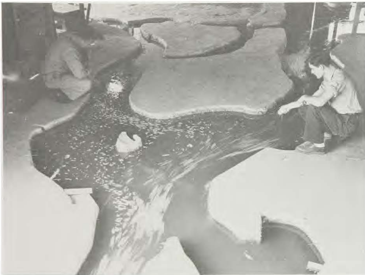
Model study of tidal currents in East River
