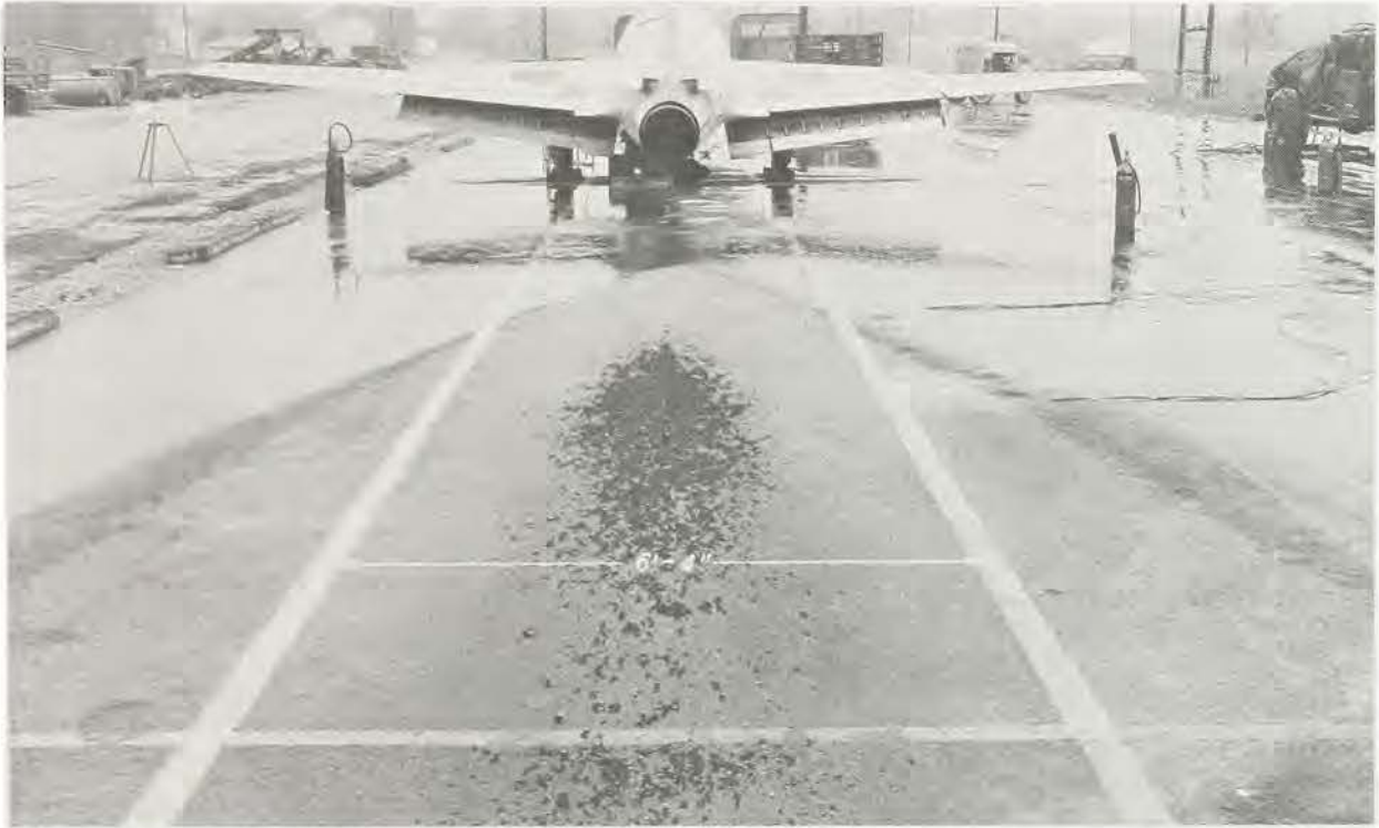
Jet plane blast test
