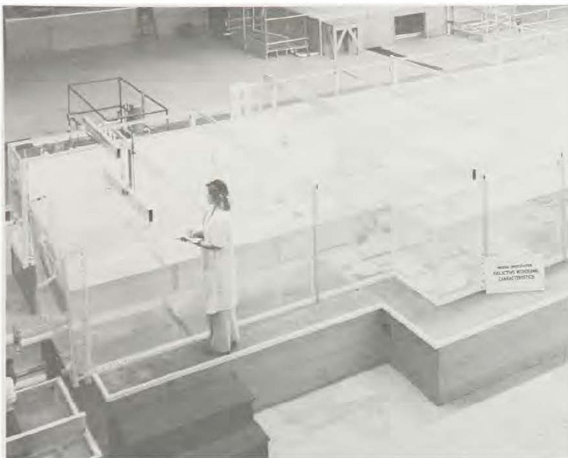
The selective withdrawal study is being conducted to improve the capabilities of the Corps to control and predict the quality of water released from impoundments
