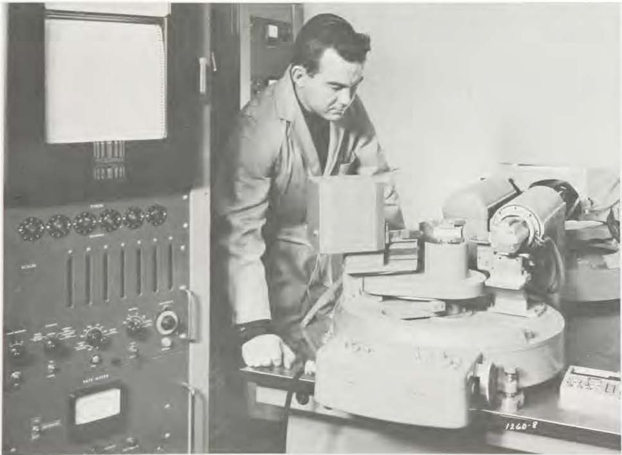
X-ray diffraction equipment with portland-cement specimen mounted in sample holder, and chart of portland cement diffraction pattern appearing on potentiometer at above left
