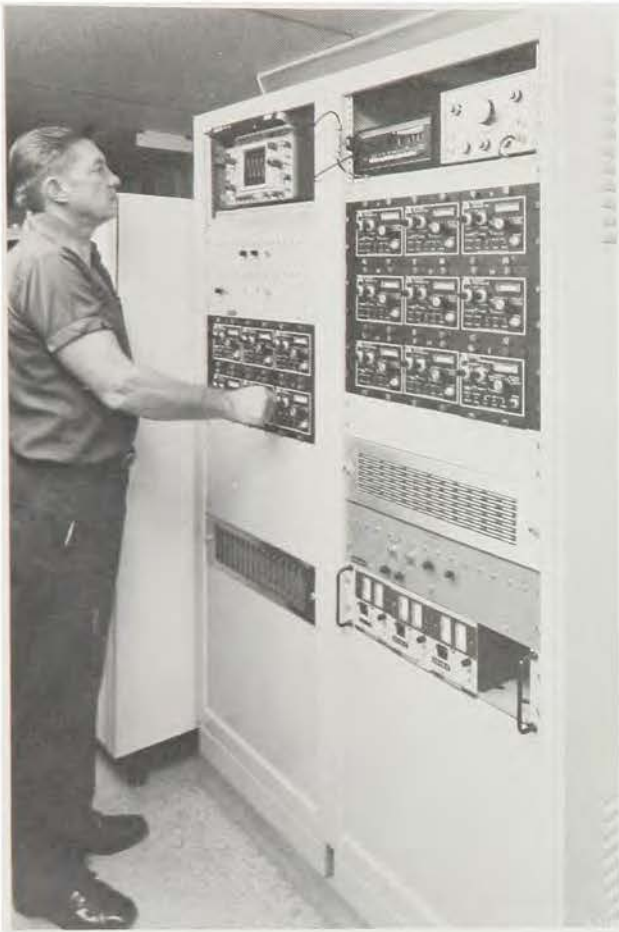
Instrumentation technician operating equipment used to control wave height, period, and phase of waves produced by a 14-section water wave generator
