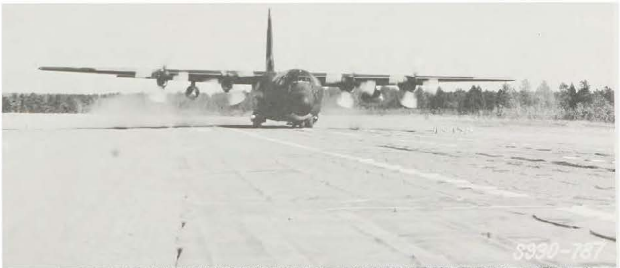
Aircraft operating on membrane-surfaced soil
