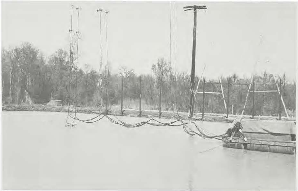
Airblast gage array used in underwater explosion tests at WES Big Black test site
