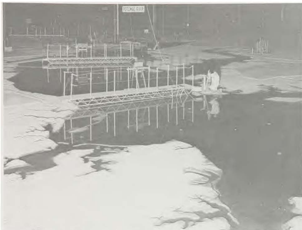
The Chesapeake Bay Model located in Matapeake, Maryland, reproduces such physical characteristics as salinity, current speeds and directions, and tides
