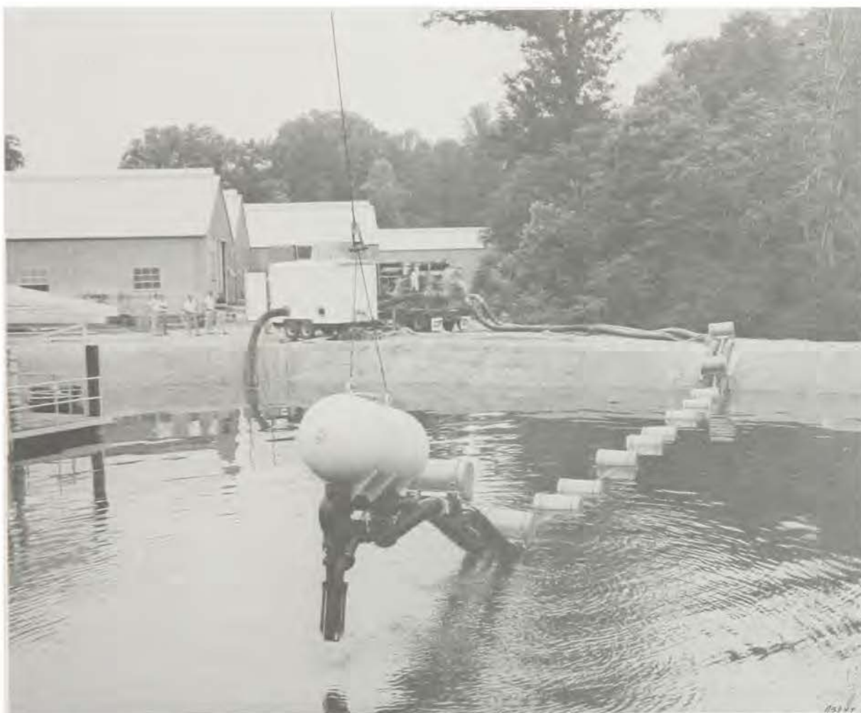
A portable sand bypassing system was developed by WES to combat shoreline erosion caused by small-craft harbor structures in the Great Lakes area. Sand bypassing is a unique method of dredging, using a centrifugal pump and a dredge pump on the shore and a jet pump in the water at the dredging site
