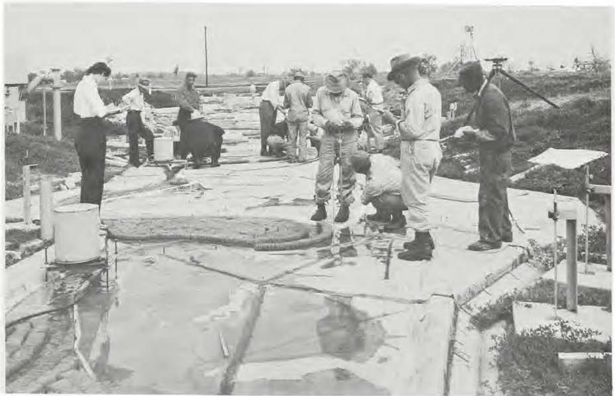
Teams taking water-surface elevations along Omaha-Council Bluff levees in the Mississippi Basin model. Circular can-like objects are automatic gages recording stages in main river channel
