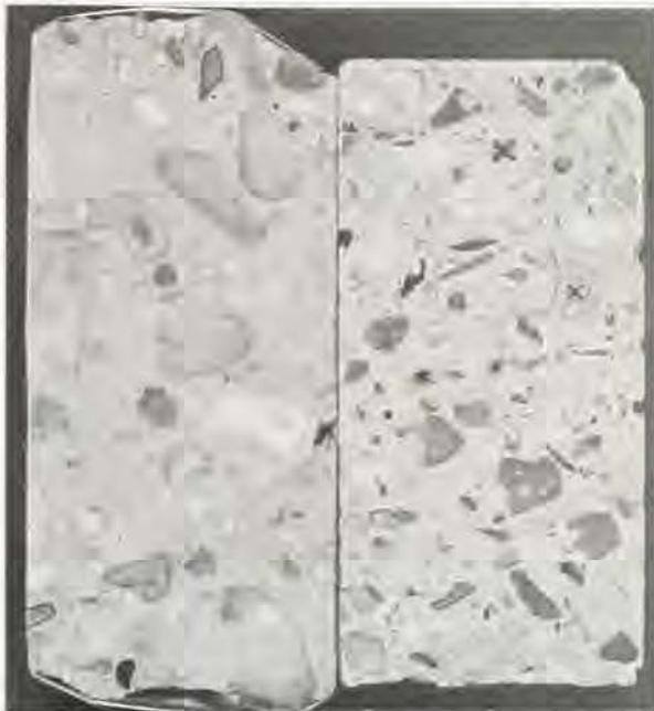
Recycled concrete. The concrete specimen shown on the right was made using discarded concrete as aggregate while the specimen on the left was made with the usual chert gravel and natural sand as aggregates. The intent of using waste concrete as aggregate is to conserve our supplies of natural aggregates and to reduce the amount of solid waste that must be disposed of daily. The specimen made with waste concrete as aggregate compares favorably with normal concrete. Based on results to date, this new usage appears feasible and desirable. The particles indicated by "x" represent fragments consisting of both mortar and coarse aggregate from the recycled concrete
