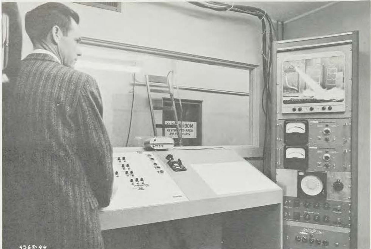
Control room for rocket motor firings with closed circuit television for observing operations
