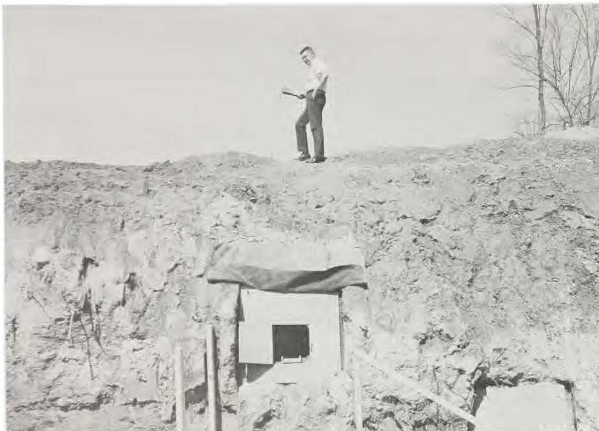
Tunnel explorer locator system, developed and built at WES, is a modified two-way communication unit capable of tracking and pinpointing the location of someone inside and also provides a two-way communication between personnel outside and those working inside the tunnel
