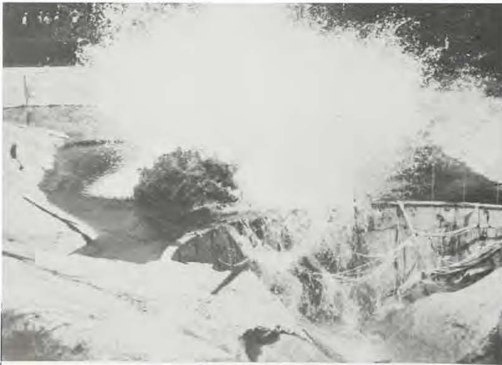
Response of the North Fork Dam model to the effects of a nearby upstream explosion
