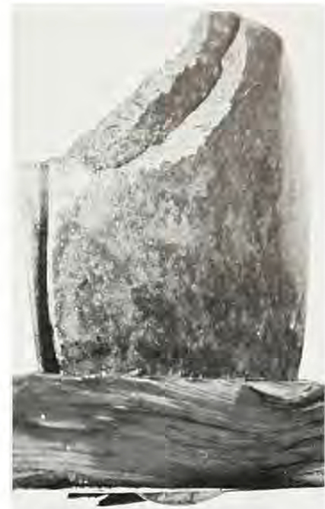
Shattered power – Hit by a speeding motor boat in Oakland Estuary, this small, one-inch thick knotty board broke two blades of an outboard motor. The blade fragments stand three inches high on the water-logged board. Between 40 and 60 tons of drift are picked up from the Bay daily by Army Engineers debris boats. The drift menaces navigation, boating and hampers industrial operations.
