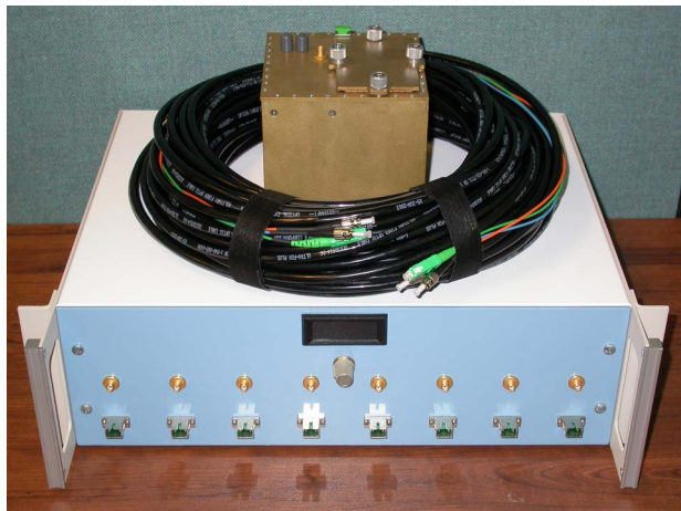
Figure 7 – Photograph of UWB analog link transmitter, fiber, and 8-channel receiver
