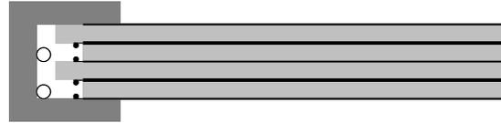
Figure 3. A side view diagram of our two-stage Stacked Blumlein pulse generator.
