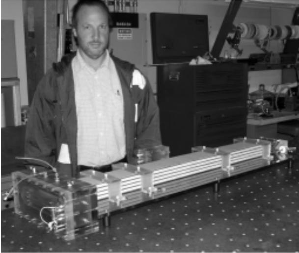
Figure 6. A photograph of the completed two-stage SBL with flashlamp illuminated spark gap switches.
