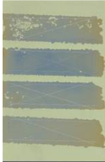
LHE Zn-Ni with MIL-PRF-85582 C1, after 4 days
