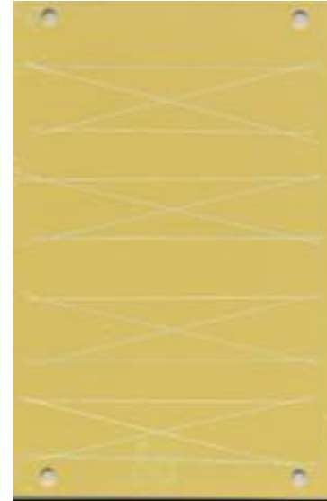
Electroplated Al with MIL-PRF- 23377, after 7 days
