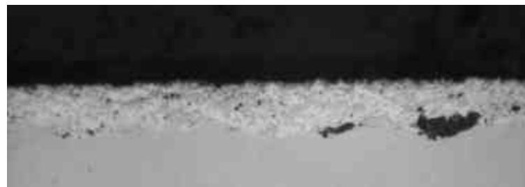
Front Compressor Rear Hub Showing Coating ~0.8 mils in Chatter Region (left) and ~1.8 Mils in Non Chatter Region (right)
