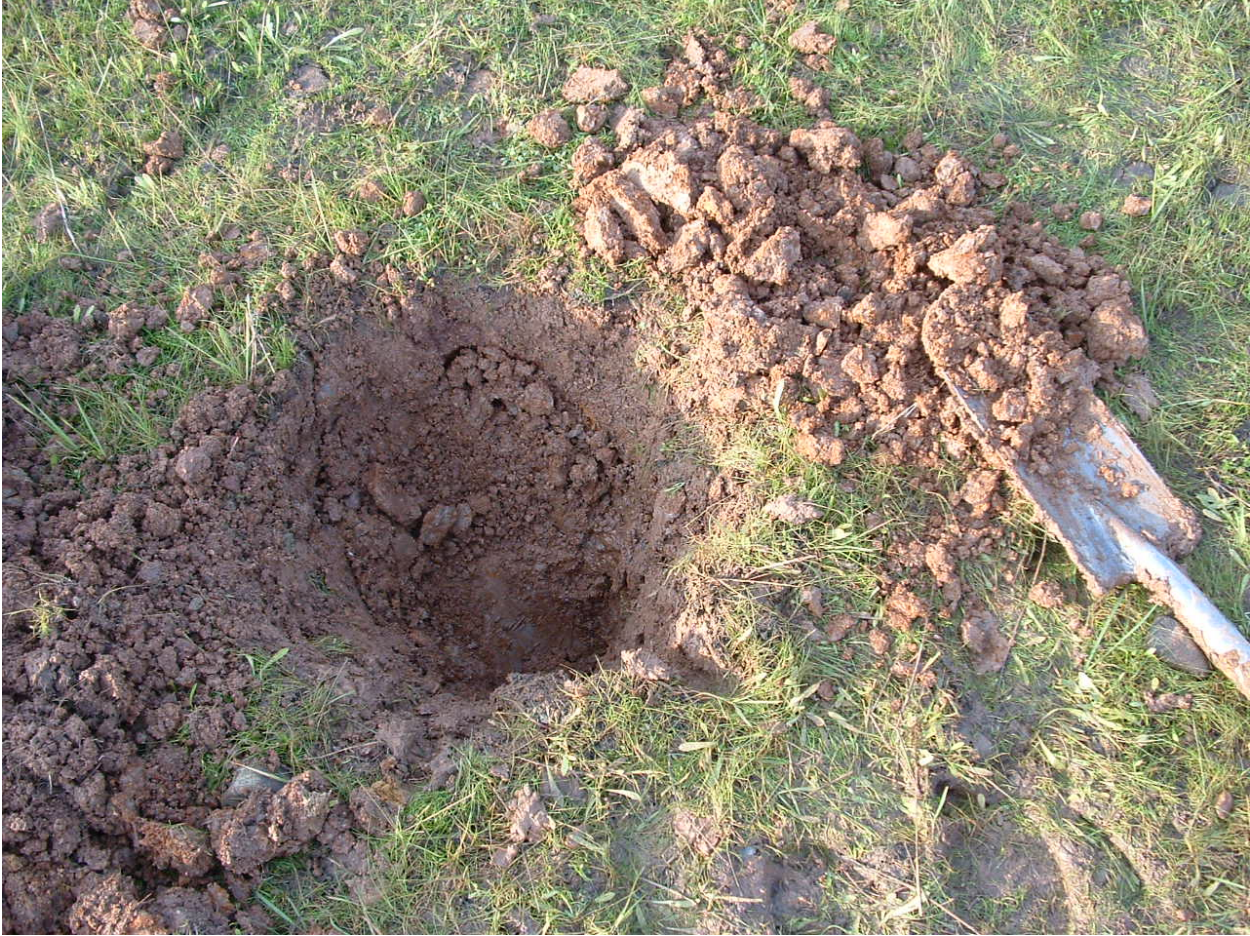
Photo 5 – Test pit (LRE-A2).
