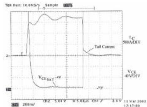
Figure 7. IGBT Dynamic Saturation and Tail Current
