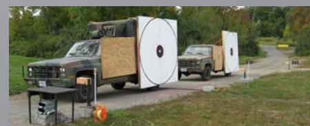
Figure 2: Convoy targets were visible during their approach to the targeting area. Shots at targets were allowed only when targets were between the white reflector posts. The pink dot on the forward truck's target constitutes a "hit."
