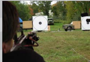
Figure 3: Truck targets were closely spaced while passing through the targeting area so the second target entered range as the first target left. Targets were available to hit for about 1.4 sec. The B.E. Meyers GBD-III-C laser is mounted on a tripod on the bed of the stationary truck in the background, and shone over the top of the first truck-mounted target.
