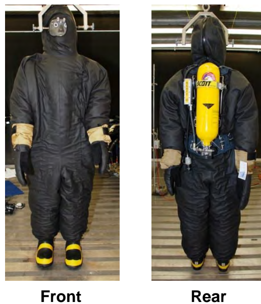
Figure 2: Prototype Steam Suit Ensemble (PSSE) on sweating thermal manikin 2
