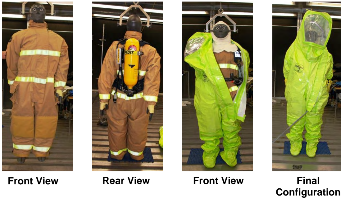
Figure 1: Submarine Steam Suit Ensemble (SSSE) on the sweating thermal manikin (Images depict donning sequence of the SSSE) 1
